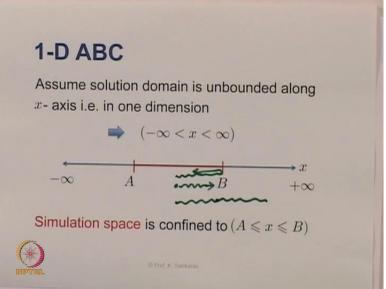
Show the ideal spaces largest space when we truncate we do not want any reflection that is going to come what I mean by reflection is assume that there is a way that is going from here to here and what happens when it reaches B is it gets reflected back so the wave that is going goes like this and gets reflected back because there is a truncation here this is a kind of adhere
