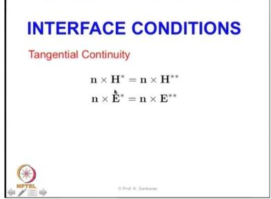
If it is a perfect electric conductor we know that the tangential component of the electric field will become equal to zero.
