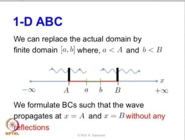
So what we are doing now is we are replacing this actual domain by a finite space so the finite space is going to be a, b and the idea is to make sure that the reflection is going to be zero at this point A and B.
