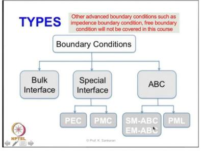
we have looked into three categories of boundary condition in that specific case we have specially looked into the bulk interface boundary condition where we talked about the tangential continuity conditions and we had looked into the special interface condition which are the perfect electric and the perfect magnetic conductor what is missing is the absorbing boundary condition itself now we are going to look into the absorbing boundary condition. (Refer Slide Time: 15:13)
