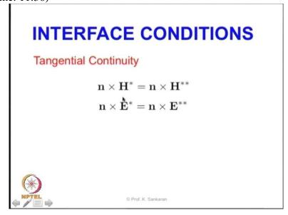
So the tangential component of the a field and H feel so in this case the left hand side and the right hand side are going to be same so this is the first interface condition that we have so in the case of special interface conditions we have to satisfy certain other conditions.
