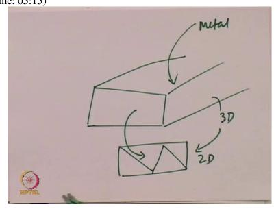
So we have a waveguide and we are trying to model this particular cross section of the waveguide so we are trying to take this particular cross-section which is nothing but this area and obviously this part are going to be the metal and this is going to be the free space where we are going to feed in certain mode and what you are trying to do here is we are going to discretise this problem so now we have converted 3D problem to a 2D problem where we are
