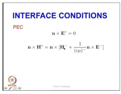
So let's look at the perfect magnetic conductor counterpart in the perfect electric conductor we have put the tangential component of a field as zero.
