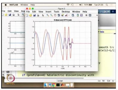
And the wave is going to stay inside the same medium x. And it is not going to emerge out in the free space. So what you see is there is a kind of a similar behaviour. The H field value is amplitude is increasing the E field amplitude is decreasing and the wave is slowing down as we expected. And it is going to slowly emerge into the medium x, but the wavelength is going to change or the wavelength is going to be reduced whereas the amplitude of H field and E field is also going to change.
