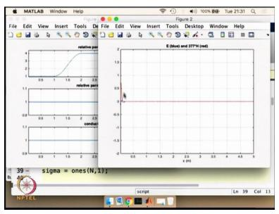
And we are trying to simulate this problem. What we are going to see is a very different kind of response. We see that the wave is trying to enter the medium. But it is not able to propagate It is getting reflected and you hardly see any impact here.
