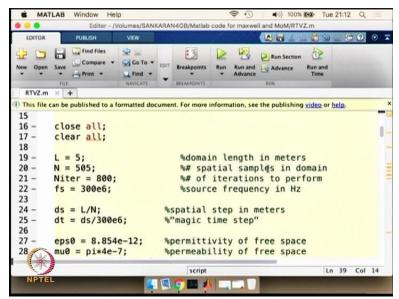
And we have set the domain length to be 5 and we are interested in discretizing this particular domain using finite difference time domain method.
