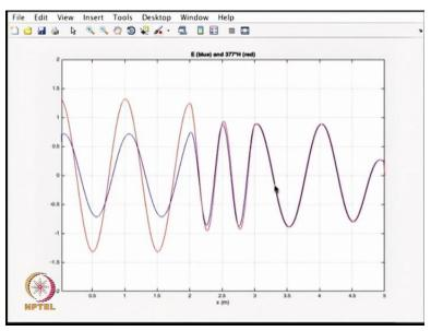
You can see the changes are quite obvious, when the wave is entering the electric field is decreasing its amplitude whereas the magnitude is increasing in its amplitude and the wavelength is changing. There is a kind of compression in the wave, and slowing down of the wave. And when it comes out it comes out in the same way.
