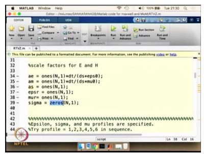
And now what we are going to do is we are going to change the value of sigma. So let us say the sigma value is going to change inside the medium that we are going to simulate. (Refer Slide Time: 22:55)
