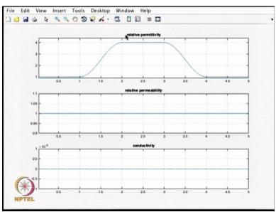
So the relative permittivity is going to be in this form and the wave when it comes inside it is getting slow down the electric field amplitude is getting increased whereas the magnetic field value is getting reduced.
