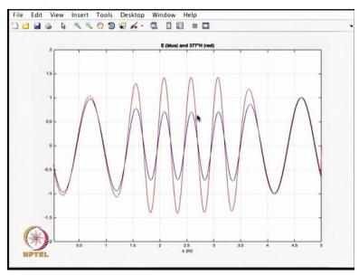
And so what we see in the case of the medium is the magnetic field value is increasing whereas the electric field value is decreasing in its amplitude. And the wave is getting slowed down and it
