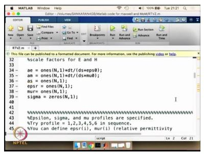
Similarly you can also derive the way for ae which is the electric term which will have Epsilon instead of Mu. And the other ones are 0 Mu r Epsilon r they are all kept to 1. Because we are talking about free space and Sigma is going to be 0 as well.
