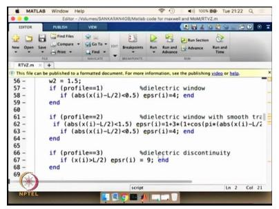
And the dielectric constants are going to also change. And the window is going to have different discontinuity. So we are going to use the value profile is equal to 2 initially and then we are going to see for other profile as well.
