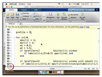
And I am going to simulate the problem for profile equal to 2 so my Mu r will be now not 1 but 2and see what is the impact of that in the particular medium that we are going to simulate (Refer Slide Time: 28:05)
