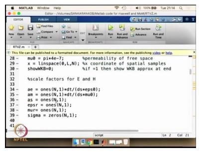
And these are the scaling factors that we are going to use for our problem so ae, am and as are going to be the terms that are going to be used in the update equation. And they follow the standard discretization where we have dt, ds and Epsilon 0 depending on the equation what we are interested in these terms are going to change.
