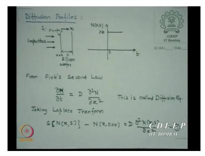
Just a minute before I show this. At t is equal to, less than equal to 0, no impurities are impinging. At t is equal to 0, the available concentration is in N0 which remains constant for all times to come. This is my initial condition which I start with and this is real life condition, that is why I did it. Is that okay?
