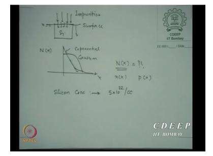
The maximum silicon concentration at a normal temperature is 5 into 10 power to 22 atoms per cc. This is the maximum carrier concentration or maximum doping, maximum atoms per cc available to you. Based on this our density recalculations we perform or rather from the major densities this number has been found. Okay, for the lattice of 8 atoms in per cell. So this is the maximum atoms, so how much doping we can do? Certainly not 5 into 10 to power 22.
