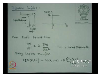
The first thing we start is now looking into profiles, that is our ultimate, that is what we are going to do, work at. So we start with profiles. First, let me say and then draw. This is silicon surface and as I say this is the depth in silicon surface, shown x, this is the silicon surface. This is silicon surface, this is silicon wafer of thickness t and t is very large compared to anything. t is, for a boundary condition what will say? t equal to infinite, means our thickness is infinite.
