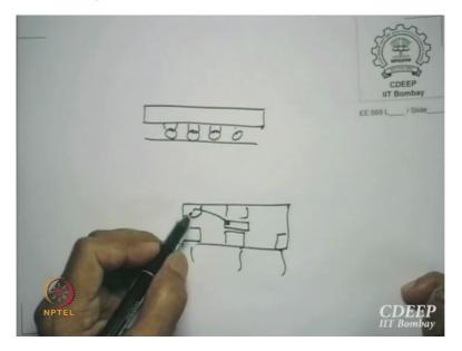
So because of that there is sufficient inductance with this. Now this inductance is used in R F and analog as an inductor itself because I need an inductor. It is variable there so it is called wire inductor. But in a normal digital circuit I do not want this to happen, okay. So I do not want this connection like this. I want flip chip. I will just bond it on balls. That is how I will use it, okay. These are all back end.
