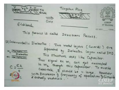
And please remember your nitride will be removed by mechanical this so there is a titanium nitride, in between there is tungsten block or plug as it is called, okay. This process is actually called Damascene process. Is that okay? How do I do it? Etch the silicon dioxide, titanium nitride, tungsten thicker, reduce thickness, do C and P to flatten it, okay. So now I have a tungsten plug which is created here. The next problem as I said, vias of course as I said by ion etching, contacts I did.
