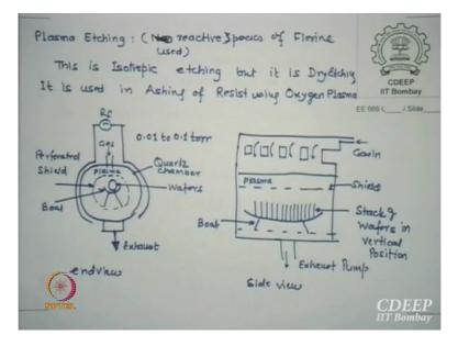
The first one we said it has two possibilities. One is ion bombardment, other is etching. So I want to create a model based on this mechanism. For R I E there are two possible mechanisms etching. One is I said related to chemical etching, the other is ion bombardment. Is that okay? Figure is drawn. This figure is also so very popular. Also you can go to applied materials lab. They have one barrel etcher kept in corner.
