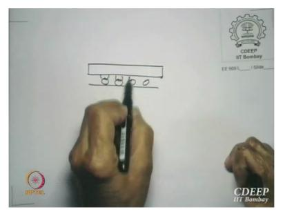
So this pad pattern is flip chipped on the ball pattern and soldered. Balls are quite thick so their inductance is very low. We are more worried about wire the way it is in a package. See this is your package patterns pads which are actually external pins and this is your chip. You have one pad, you wire bond here. Now this length is not very small.
