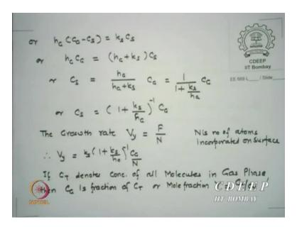
So if I equate them and collect the terms, I can write CS is equal to HG upon HG + KS into CG 1 upon 1 + KS by HG into CS, or in a 1 + KS by HG to the power - 1 into CG. So I now related CS and CG through what terms? Mass transfer coefficient and reaction rate constant. The growth
