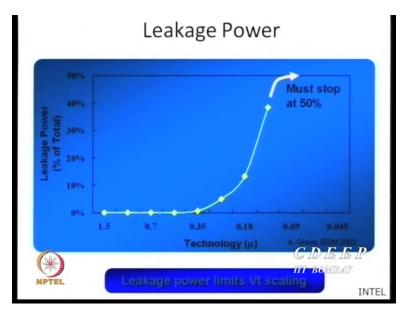
By speed I already said videogames nothing else. This is some kind of statistic from Intel many years ago this is leakage current and one can see 50 percent of the, is already reaching as a leakage path, okay. So we are worried that latter as I say in 30 nanometre down technologies off current were 66 percent. So why do a circuit which is losing power without doing anything, okay but that is the game.
