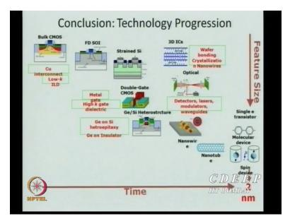
We went from bulk CMOS, we went for fully depleted silicon SOI silicon on insulator devices, strained silicon, we are looking for high k which is called double gate FET which is very first better MOS transistor created, we can make few more gates will it is called trigates, triple fin gate or multi-fin gates which is what Intel is working, so these will give better performance compact to because there is a problem which I never said.
