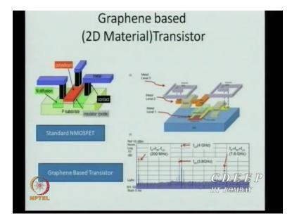
This is a normal mass transistor and this is Graphene has a small film below, so there is electron moves through the Graphene area their conductivity is very very high typically it could be infinite also in ideal state, so huge currents can actually flow no on resistance, okay. So it can be very high speed device this is what is being tried. So we are working for a, I do not know whether you are.
