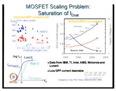
As I say as I start scaling, in the case of on currents if a MOS transistor the RV characteristics is thing like this, okay. Now one can see from here, one believes the of current below threshold is very small but if you scale even this current of 0 Vt or small vt the current is very high. So of current, of current means the transistor is switched off officially, input Vg is smaller than Vt but there is a current, okay.
