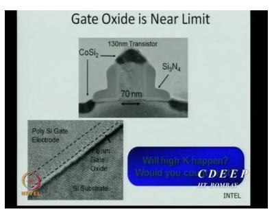
This is something which in 2000 it right and I will show you the latest one, we were trying to state that if I start scaling the dimensions of the oxide thickness of your mass transistor also scales down. So for example scaling long to say 22 nanometres or even lower the oxide thickness required is less than 5 angstrom, half nanometre. Now if your oxide thickness is half nanometre all over its called thickness of the oxide or insulator.
