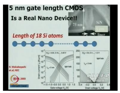
Just look at this 5 nanometre gate length CMOS is a real nano device, okay. It has a length of 18 silicon atoms, okay. You can see around and in 2003 itself this device was made, so it is not that one is not able to make lower technology node but if I make millions of them only to3 may work
