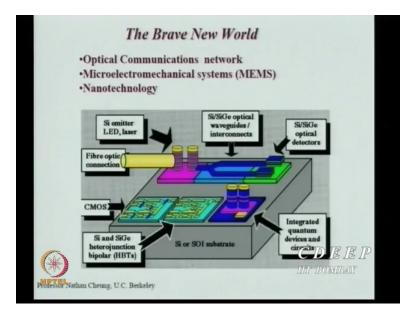
However humans are great we are now looking for a Brave New World which has come from Professor Nathan from Berkeley. Can see every kind of system can be built on silicon substrate, okay. You have CMOS devices, we have silicon germanium heterojunction devices, we have fibre optics connection, we have silicon LEDs, we have silicon germanium optical waveguides, we have silicon germanium optical detectors and we have quantum dot-based devices, okay.
