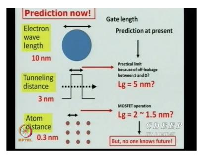
As you scale down the thickness of channel I am in this, sorry gate thickness one can see that we always thought electron does not have energy enough to cross but there is a possible lady of tunnel, okay. Because of variety of effects, 3 nanometres you do it will just cross, okay. Then there is atomic distance 3 angstroms, what else? 2.6 1 is the minimum (()) (48:23) that's it, so you cannot put less than an atom otherwise what you will do? However all said and done but no one knows the future.
