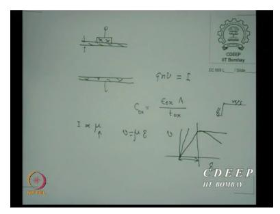
We have the (()) (53:28) Intel works, Intel has been working on process which is called one of the major interest in high-speed was if you look at it one of the most important current is I is proportional to mu in MOS transistors Ids is proportional to mu c ox, okay. So the speed is limited by available mobility. So in silicon are given high fields it may be around typically 600 centimetres square per volt second is highest ability one can get in a MOS structure.
