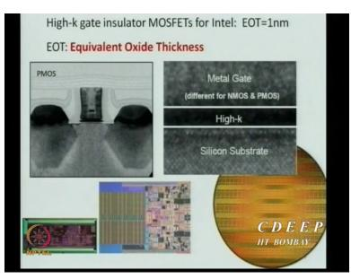
This is what high K looks like actual devise which was made in TIT and we have a metal gate instead of silicon gate which also is another change in technology and this is a high K based design, it has a small 4 bit microprocessor which has a bank of SRAMs, okay. This has an EOT of 1 nanometre.
