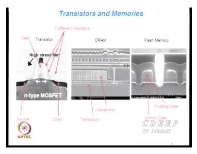
The semiconductor technology has 3 driving forces and these are 3 ones which you will hear, the first of course is the transistor technology, transistors are used in mostly in logic as well as analogue RF systems, from these major transistors you make there are other technologies which is driving semiconductors now, one is of course the memory technology DRAM technology as it is called and all of you know how much DRAMs are now available.
