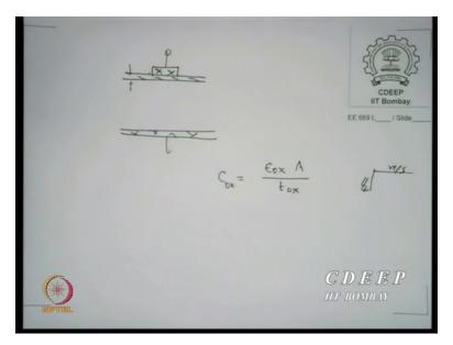
So I made a take back what I did is, I said fine I cannot scale down as then say 10 nanometres out of this one nanometre, so I did something like this, this is my capacitor, this is my insulator, this is my gate, this is a standard capacitor, this is a mass capacitor, the capacitance of this oxide whatever it is Epsilon ox ks Epsilon 0 multiplied by area divided by oxide thickness.
