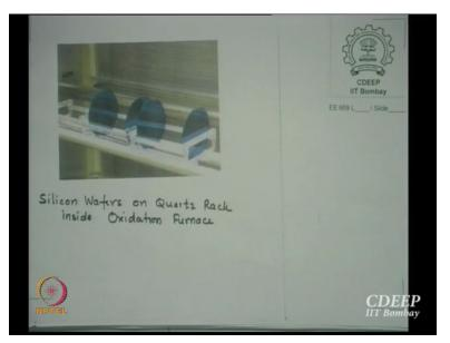
Typically if you see a rack, these silicon wafers are mounted in a quartz rack, you can see they go vertically down and they fit it into the slots. This is how the rack there, so larger the rack size, larger is the number of wafers one can introduce inside. So any number of wafers you can load depending on the temperature, central temperature zone you have wider or smaller and the rack size you have.
