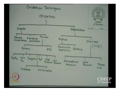
So there is a possibility, this is no different from furnace. All that you are doing is temperature is created in a different way. In furnace we can have dry oxidation, we can have wet oxidation and we can also have another one which I will show my results on that, pyrogenic. Then we can use oxide, N2O oxides. Then we can have high pressure oxidations, we can have low pressure oxidations.
