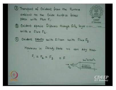
So oxidant reacts with silicon with flux F3. However in, there are two things we say in devices as well as in any process for that matter, thermodynamic process. There are two terms which we use, thermal equilibrium and steady state. What does that say? In the case of thermal equilibrium as there is no external force applied. The system is only by thermodynamically adjusting its energy to the minimum. This is the entropy, this relationship.
