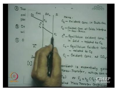
And the third before I come back again, it reaches silicon surface or silicon-silicon interface and reacts with silicon to form new oxide.
