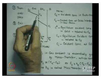
The oxidant specie then before we, this word, it has already impinged here. Then it gets inside SiO2 by the process of diffusion because there is no oxidant here. There is oxidant here, there is a gradient creation. So oxidant specie diffuses in the SiO2 to reach silicon-silicon dioxide interface.
