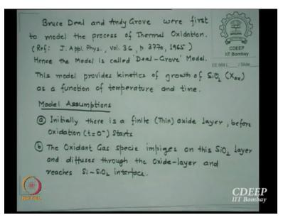
So I come back to this. So as I just now said, initially there is a finite thickness, yes, initially there is a finite thickness. Oxidant gas specie impinges on SiO2 layer.
