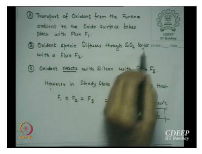
So the second flux is diffuses through SiO2 with a flux F2.
