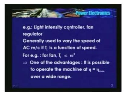
Where are they used? They are very popular in fan regulators, light intensity controllers. I have told you that if the induction machine is driving a fan type of load, the speed can be varied over a wide range by varying the magnitude of the input voltage frequency being the same. The type of load is fan type of load wherein  $T_L$  is proportional to omega square. What is another advantage? It is possible to operate the machine at maximum efficiency over a wide range.
