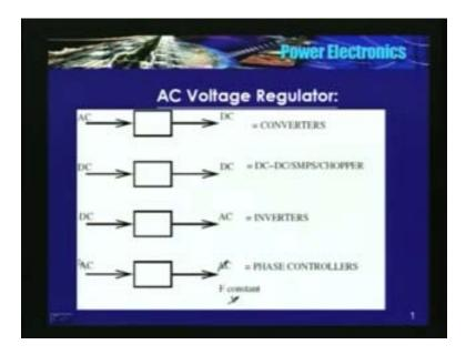
See here, we are here; input is AC, output is also AC. Frequency constant, variable voltage. They are known as AC voltage regulators AC voltage regulators.
