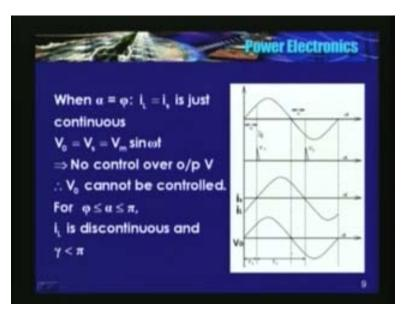
See here, trigger angle alpha is equal to phi, current is sinusoidal. Now, current is sinusoidal. That means either it has to flow through either  $T_1$  or  $T_2$ . So, you will have the input voltage is same as the output voltage. The output load applied voltage to the load is sinusoidal and it is equal to the input voltage  $V_i$  itself.
