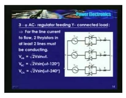
Let me tell you one thing; analysis of 3 phase AC voltage regulator is bit difficult compared to a 3 phase AC to DC converter. So, that is a reason I will use a resistive load. I will not analyze the circuit for a RL load. So, this is the possible configuration; AN BN CN are the phase voltages, a 3 phase resistive load, star connected and you have 3 pairs of back to back connected SCRs.
