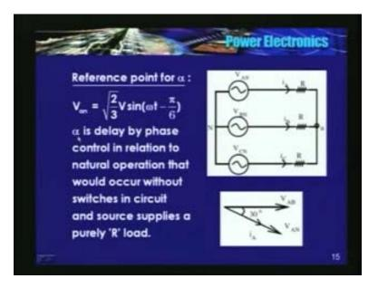
Now, what is the reference point for alpha or where do I start measuring alpha from? What did you do in 3 phase AC to DC rectification? We took the point of natural commutation as the reference point. Now here, the reference point is taken as I will show you, see, here it is mentioned alpha is a delay by a phase control in relation to the natural operation that would occur without switches in circuit and source supply a purely a resistive load.
