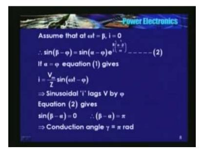
Now, see this is the equation. Assume that at omega t is equal to beta, i will again become 0. So, you substitute this condition in the previous equation. So, what do I get? You will get sin beta minus phi is equal to sin alpha minus phi in this term. Now, if alpha is equal to phi, in other words, if the trigger angle is same as the power factor angle, what does the equation 1 say? It says that this term will become 0.
