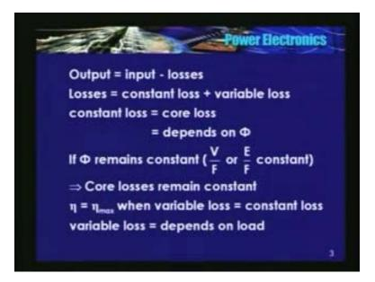
How is that possible? Let us see here. We all know that output is equal to input minus losses. Now, what are the losses? There are 2 types; one is constant loss plus the variable loss. Constant
