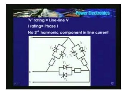
Now, when the load is connected in delta? This could be one of the configurations. Again, back to back 3 bands; these are 3 loads, they are connected in each phase. What happens here? The current through the SCR is the phase current but then the voltage is the line to line voltage. But then you will not have third harmonic current in the line. In the previous case, because there is a neutral you will have third harmonic currents in the line. But in a 3 phase 3 wire system no triplen harmonics.
