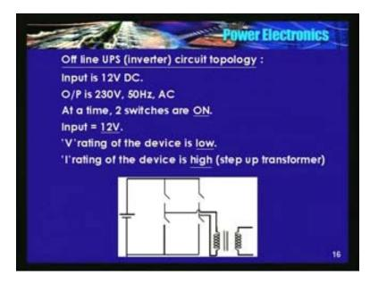
Now, let me talk about an off line UPS or an inverter, circuit topology. Why I am calling off line UPS is the inverter that we are that used in our home; the moment AC supply goes, after some time say, after a fraction of a second also, the inverter comes in. So, that is why I am calling a off line UPS.
