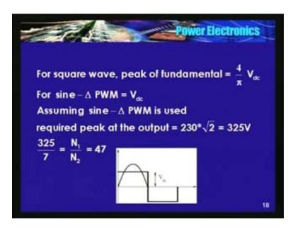
Now if I use a square wave operation or if I if the device are on for 180 degrees, the peak of the fundamental is 4 by pi into  $V_{dc}$ . See here, I have a if I if I take 180 degree conduction; this is  $V_{dc}$ , the peak of this is 4 by pi into  $V_{dc}$  and if you want a pulse width modulated inverter because square wave has a higher frequency components. In the single phase case; 3, 5, 7 all are odd harmonics.
