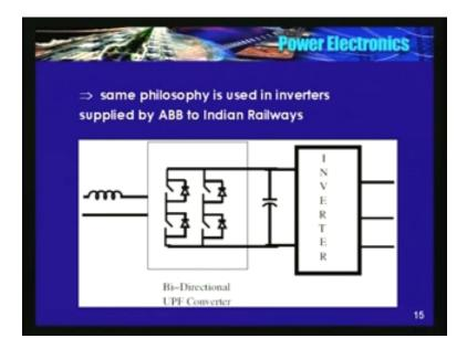
We call it as a unity power factor converter. I am just showing a single phase inverter, single phase. We have 4 control switches, may be see freewheeling diodes, capacitor voltage, here
