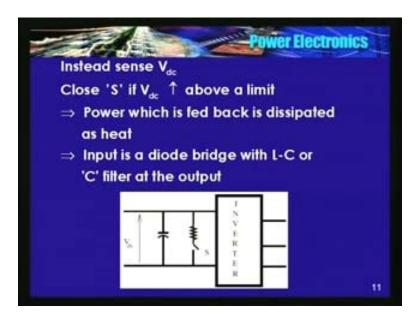
So, what has been done is if this  $V_{dc}$  is sensed and the moment it increases above the set value, use this S, the switch is closed. So, what happens? The capacitor discharges or this energy, the additional energy that is got or received from the load is dissipated as heat. So, since  $V_{dc}$ ; the moment it crosses the set value, close this, dissipate the energy in the resistor and when it falls to below a certain value, open S.
