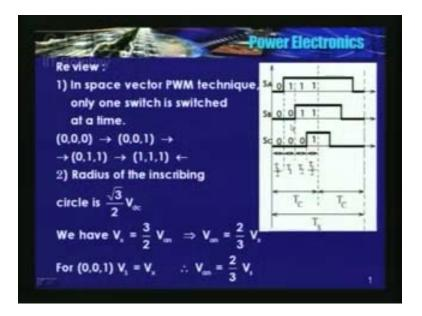
So, vector  $V_1$  is applied for  $T_1$  duration and at the end of  $T_1$ , we turned on the upper switch of phase B. See, we did not do anything to the upper switch of phase A, it is still on. We turned on another switch and upper switch of phase C is still off. So, it is 011. We call this vector as  $V_2$  and that is applied for  $T_2$  duration and at the end of  $T_2$ , we turned on the upper switch of phase C.
