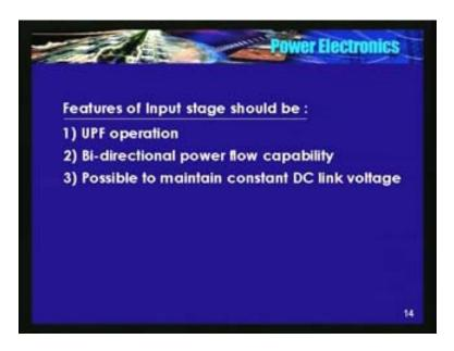
So, if I summarize; the features of the input stage should be unity power factor operation, bi directional power flow capability and possible to maintain constant DC link voltage. So, these are the features that input stage should have. How will you achieve? See here, you have studied this, this converter.
