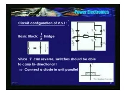
A half bridge configuration, half bridge, a basic building block. We have a center tapped DC source,  $V_{DC}$  by 2,  $V_{DC}$  by 2, 2 switches  $S_1$  and  $S_2$  and load is connected between the centre point of the voltage source and the centre point of these 2 devices. I will just repeat; I might have done this in AC to DC conversion and I represent a switch in this fashion. When I close the switch, current flows in this fashion, current flows in this fashion.
