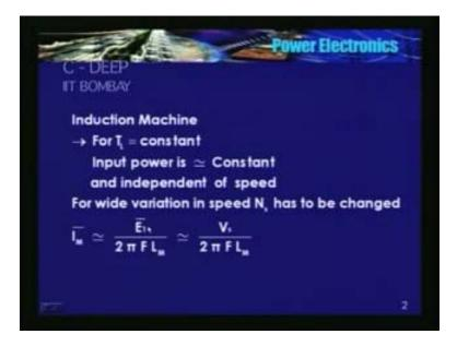
So therefore, see in this equation, magnetizing current is given by  $E_1$  divided by 2 pi F into  $L_M$ . Actually, it is not approximate, this is equal.  $I_M$  is equal to please, this is equal to  $E_1$  divided by 2 pi F into  $L_M$  which is approximately equal to  $V_S$  divided by 2 pi F into  $L_M$ .
