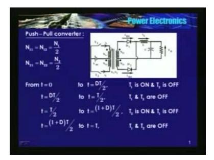
I will use a center tapped winding; see the dotted polarities and I will connect the supply here and 2 switches  $T_1$  and  $T_2$ . So, when I close  $T_1$ , current enters the dot, so direction of flux, whereas, when I close switch  $T_2$ , see, current leaves the dot leaves the dot. So, whatever that happens in  $N_{11}$  happens, the just the opposite in  $N_{12}$ .
