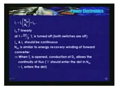
Therefore,  $i_1$  is the load current. This  $i_L$  is flowing in  $N_{21}$ , this  $N_{21}$  is nothing but  $N_2$  by 2 but whereas,  $i_1$  is flowing in  $N_{11}$  and  $N_{11}$  is nothing but  $N_1$  by 2. So,  $i_1$  is equal to  $i_L$  into  $N_2$  divided  $N_1$  plus the magnetizing current.  $I_M$  increases linearly.
