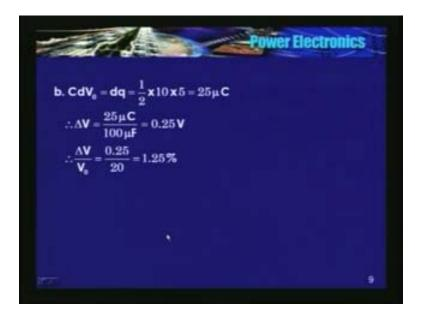
And, the same procedure to determine the output voltage ripple; C  $dV_0DT$ should be equal to dq is equal to half. See, area of this angle. This is DT by 2 because entire DT is 4, this is linear, so this is this point is DT by 2 DT by 2 or midpoint in between 0 to DT and this is the midpoint between DT and T.
