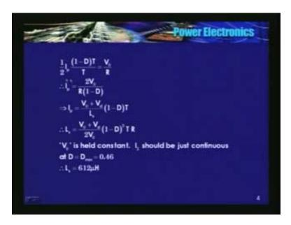
So, this is the equation; average  $i_2$  should be equal to average  $i_0$ . So, the peak value of the current is given by this equation, Now, from this figure I know the slope, I know this time period. So, I can calculate this current, this value. I know the slope, I know this period; I can calculate this current.
