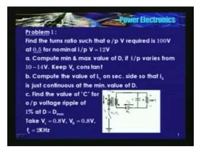
So, first one is on fly back converter. The problem states that see, required output voltage is 100 volts and nominal input is 12 volt, input is 12 volts. So, the the problem says find the turns ratio such that output voltage required is 100 volts at D is equal to 0.5. See, generally the nominal value of the D is around 0.5, even for fly back as well as as well as the forward converters, at 0.5 for a nominal input voltage of 12 volts. See, input is 12 and output voltage is 100 volts.
