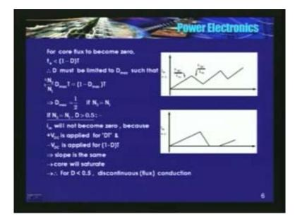
So, if D is equal to  $D_{max}$ , this is the relationship. I will choose  $N_1$  is equal to  $N_3$  number of turns in both the windings is the same. So, I will find that maximum value of D is 0.5 maximum value of D is 0.5. In a forward converter, if the number of turns in the tertiary and the primary is the same, the maximum value you can go is 0.5. Can you go or is it possible to go above 0.5 or what happens if I increase D above 0.5?
