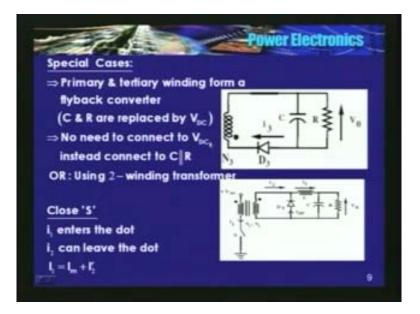
See something like this;  $N_3$  coil, diode  $D_3$  and C and R. This is nothing but a fly back convertor. I have not shown the primary here, primary does exist primary does exist because see here, in the previous see, this current is entering the dot here, current is entering the dot in the primary. So, for a flux continuity, the tertiary current also should enter the dot current also should enter the dot.
