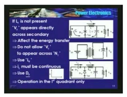
What is what is the third case? What is the third case? The third interested case is there is no LF at all. Do not use LF, do not use LF, do not use LF. Just because we had used LF, we wanted we connected a DF here because when I open the switch, this current has to be continuous. So, it will start flowing through DF. So, if there is no LF, you may not even require this DF. But then what will happen?
