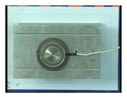
So, now you can see the progress in a power semi conductor technology. A small transistor relatively higher, two 75 ampere devices, six 75 amperes devices, there are six diodes, anti parallel diodes. Here there are two anti parallel diodes, 300 ampere device,
