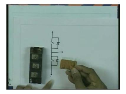
See another, a very recent power module, what it is? See here, there are three such legs if I consider this is one leg, there are three such legs here. Each device can carry again 75 amperes and it can block 1200 volts. The rating there are 6 such devices integrated
