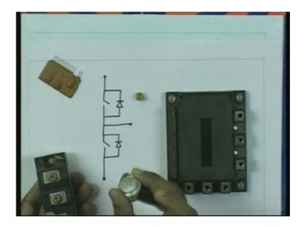
See, there is another very high power device again a controllable device. Can carry 300 amperes of current, can block again 1200 volts, two sides. Now, it requires two heat sinks, some sort of a sand witch type. Again you require one more heat sink on top of it.
