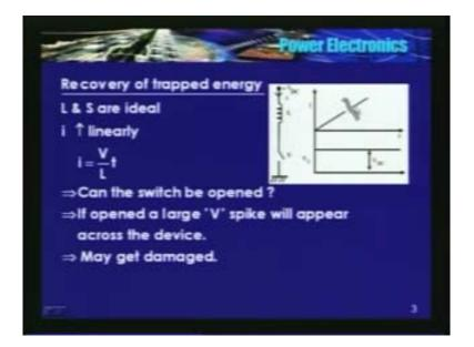
Consider this circuit; L is ideal, switch is also ideal. Close the switch or DC supply is applied to an inductor. So therefore, current will increase linearly. Inductor is not saturated, so current increases linearly. After some time, I want to open the switch. Can I open the switch now? Answer is no.
