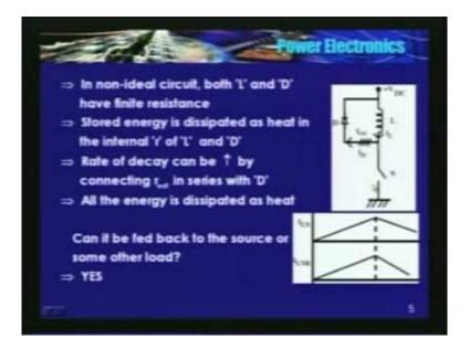
Since this resistance is small, the decay of current is also very small. The current decays very slowly. See in this fashion, decays very slowly. So, you may close the switch next time. At that time, immediately, whatever the current that is flowing through the diode starts flowing through the switch. So, if I close the switch somewhere at this point, this current, the magnitude of this current or the magnitude of current that was flowing through the diode starts flowing through this switch.
