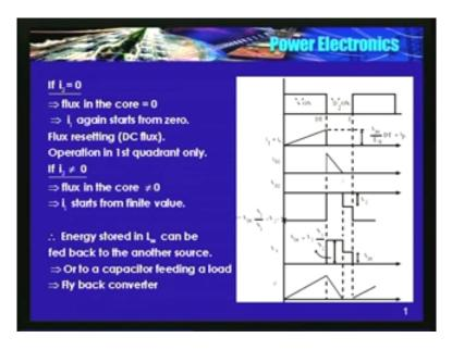
See here, S is on,  $D_2$  is on. When I open when I close S or during 0 to DT primary current which is also the source current which is nothing but the magnetizing current increases linearly. Now, why is it starting from 0? It starts from 0 because in the previous cycle, just prior to closing S,  $i_2$  is 0. I will repeat; it starts from 0 because just prior to closing S or much before closing the switch S, current in the secondary has become 0.
