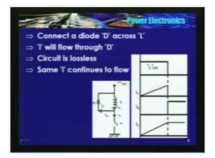
I connect a diode across the inductor. This diode is also known as freewheeling diode and sometimes we can call it as fly wheel diode, remember. Why fly wheel? You know that fly wheel stores the energy when it is accelerated and when it is decelerated, what happens? It is it can supply the energy back to the load, fly wheel concept.
