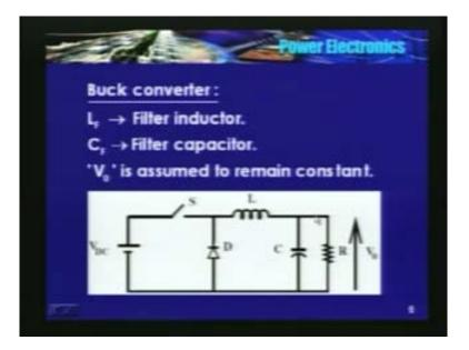
Now, the first one in switch mode power conversion or DC to DC conversion is the buck converter, a buck converter, a buck. Input is DC, output is available at this point, I am assuming that a resistive load is connected at the output, R, C is the filter capacitor sorry CF, it should be CF, is the filter capacitor, LF is the filter inductor, LF is the filter inductor, D is the freewheeling diode, freewheeling diode. S is the switch, S is the switch, what sort of a switch?
