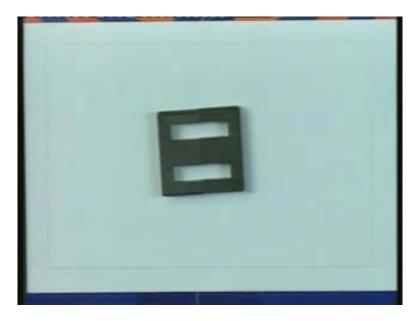
This is a ferrite core. So, here we see, this is a ferrite core, lamination for a sorry core for a ferrite transformer made up of, this material is of ferrite. I can use it for an inductor or I can use it for a transformer. It is very brittle. So, laminations, you cannot make thin laminations out of it. So, what is the average flux density in this core? It is again is low, is of the order of maybe, 0.2 to 0.25. Designer will take of the order of 0.2 to 0.5.
