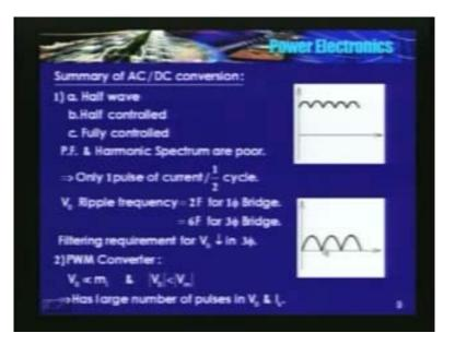
I hope you remember, for alpha is equal to 0, a 3 phase uncontrolled bridge. This is for alpha is equal to 0 for a single phase bridge. So, if I want to have a constant DC, I need to have a very small capacitor here because this voltage approximately constant. This is root 3 times, this is 1.5 times, approximately comes 1.5 to 1.713, whereas, this varies from 0 to  $V_m$  and I want a constant value. So definitely, filtering in this case is minimum, is much more than this.
