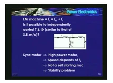
See, in this equivalent circuit the rotor current, equivalent rotor current and magnetizing current, vector sum of these two is a stator current. So, whatever that happens in the rotor circuit will affect the magnetizing current and therefore the stator current. In DC machine? Yes, the rotor current and field current, they are always at 90 degree. So, we could control them independently.
