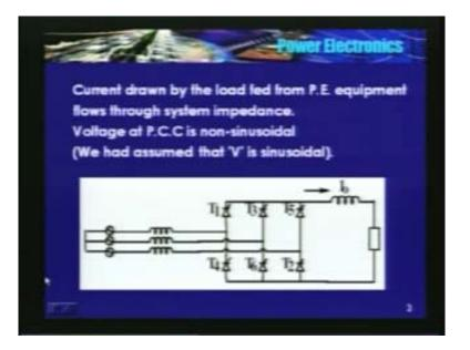
Here is the 3 phase bridge, pure sinusoid. I have neglected the resistance here. I am assuming load current should be constant and ripple free. So, each device conducts for 120 degrees, source supplies power for 240 degrees. If I assume  $I_0$  to be constant and ripple free, source current is going to be a square wave.
