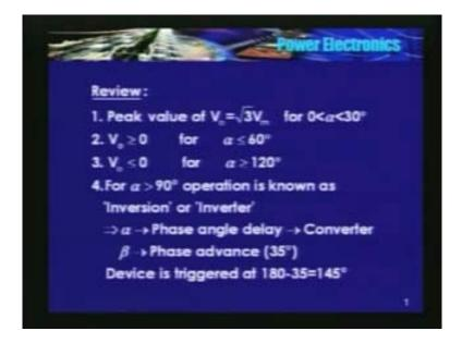
Instantaneous value of output voltage is either 0 or negative for alpha greater than 120. For 120 degrees, it just becomes 0 and it becomes negative. Therefore, to start the bridge or to energize the bridge, alpha should be less than 120 degrees. You can establish a current in the bridge only if alpha is less than 120 degrees, remember this.
