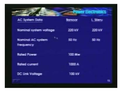
See, here is the technical data. Nominal voltage is 220 KV, both frequencies are 50. Nominal frequency is 100 mega watts, rated current is 1 kilo ampere, DC link voltage is 1000 KV. This is unit 1. Barsoor to lower Sileru, stage 1. That is about HVDC.
