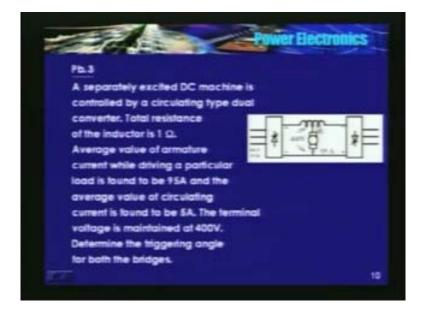
So, here is another very educative problem, 3 phase dual converter feeding a high HP motor. May be, a HP rating may be of the order of 100 HP, 400 volts. Total resistance of the inductor is 1 ohm. So, you have 0.5 ohms this side and 0.5 ohms this side. At a particular load current, this current is found to be 95 amperes and the circulating current, average value of the circulating current is 5 amperes.
