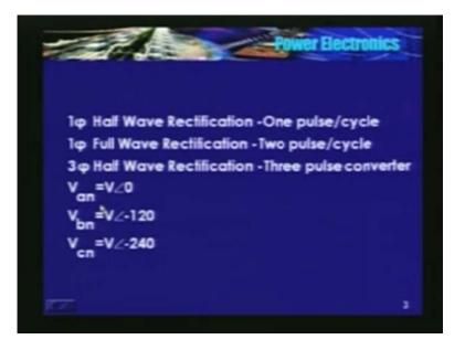
So again, things are bit difficult. You need to understand because so far there was only single phase voltage,  $V_{an} V_m$  sin omega t. Now, there are 3 voltages which are displaced by 120 degrees. Magnitude may be the same.
