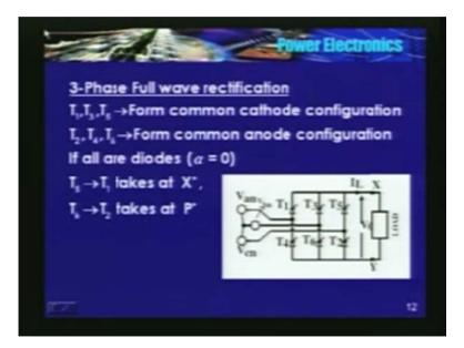
Again, 3 phase half wave rectification has a DC component. In the single phase case, from half wave rectification we went to full wave rectification. Same thing we will do in a 3 phase, full 3 phase circuits. Remember, it is going to be a bit more difficult. Here is the bridge,  $T_1$ ,  $T_3$ ,  $T_5$  form a common cathode configuration,  $T_4$ ,  $T_6$ ,  $T_2$  form a common anode configuration.  $V_{an}$ ,  $V_{bn}$  and  $V_{cn}$  are the input voltages.
