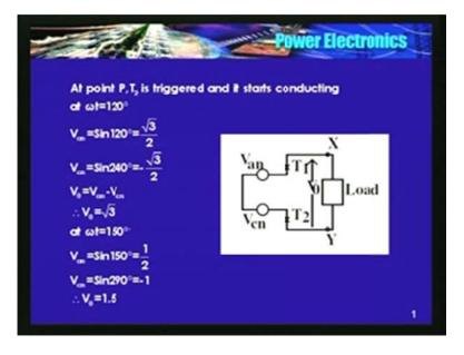
So, what is the value? It is, sin 60 is root 3 by 2, sin 300 is minus root 3 by 2. The load voltage is  $V_{an}$  minus  $V_{bn}$ . It is root 3 times the peak of the input voltage or root 3 per unit. So, if you see here, it is root 3. It was 1.5 that is at alpha is equal to 0 or omega t is equal to 30 degrees with respect to the positive 0 crossing of phase A, after 30 degrees, the peak value of the output voltage becomes 1.73 times.
