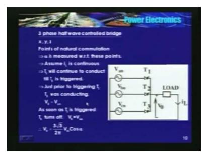
So, that is about half wave uncontrolled bridge. Change over from 1 device to another device takes place at X, Y and Z. At point X, point Y, and point Z, instantaneous value of 2 phases is the same. Since, change over from 1 diode to another diode takes place at these points, they are known as point of natural commutation.
