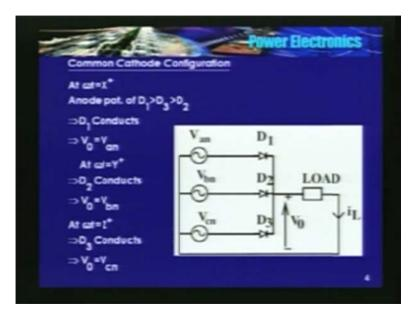
So, here is a bridge, the 3 diodes, first we will do uncontrolled, they form a common cathode configuration and load is connected between the common cathode and the start point. 3 diodes,  $D_1 D_2 D_3$ , they form a common cathode configuration. Therefore, the diode whose anode potential is at rest will start conducting.
