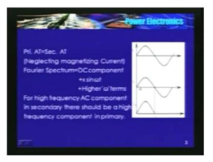
The secondary voltage, output voltage across R. Load is purely resistive, current wave form is also half wave rectifier. So, current flows in the load, remember, current flows in the load from 0 to pi. The expression is given by secondary sinusoidal voltage divided by r that is if I say some x into sin omega t, so expression for i is x into sin omega t divided by r and from pi to 2 pi, current is 0.
