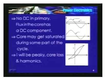
So, flux in the core has a DC component, phi DC and a sinusoidal component. This flux is produced by the magnetizing current. So, flux in the core is phi DC plus phi fundamental. So, I have a waveform, a sinusoidal waveform having a DC shift or DC bias. What is the effect? What is the consequence? What will happen if there is a flux, a DC flux in the core?
