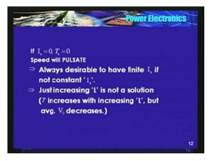
Just by increasing L, we found that gamma may be increasing but then, load voltage, the average value of the output voltage decreases. So just by increasing L, may not be a solution for these circuits. What next? Is there a way out? I think so, there is a way out. What is that?
