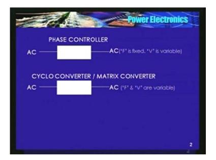
The fifth one, the fourth one: input is AC, output is also AC but the frequency of the output voltage is same as the input, whereas, the magnitude is changing. These are known as phase controllers. They are often used in fan regulators, you might have seen. A small regulator, just by changing the knob you are varying the speed. They are basically phase controllers.
