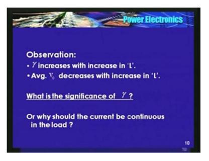
What are the observations? We found that when gamma for a purely resistive load, diode conducts for pi by 2 radians. Sorry, diode conducts for pi radians. When the load is purely inductive, diode conducts for 2 pi radians and for a RL load, diode conducts for durations greater than pi. So, gamma increases with an increase in L. But then, average value of the output voltage decreases with L. Why? Because beyond pi, we are applying a negative voltage to the load.
