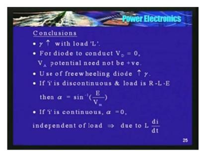
So, what are the conclusions? First 1 is the conduction angle or the duration for which diode conducts increases with load inductance. Second is for the diode to conduct, voltage across the diode should be 0. It is not only the anode potential alone will decide the conducting state of the diode, it is also the cathode potential, it is also the cathode potential will determine whether that diode can conduct or not.
