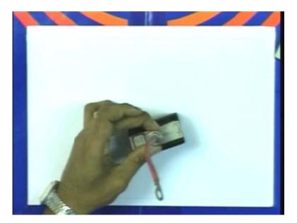
So cathode, anode: body is anode, this is a cathode. It is a 2 element device. These are known as the uncontrolled device: hence the name, uncontrolled rectification. Let us see, what are the various parameters?
