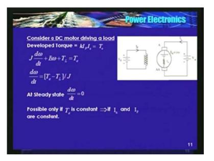
Consider a simple case, I have a DC motor, torque equation is K into phi into  $I_A$  and the equation is J d omega by dt plus B omega plus  $T_L$  is equal to  $T_e$ .  $T_e$  is the torque developed by the motor, load torque, frictional torque, J is the moment of inertia. So if I neglect the frictional torque, d omega by dt is equal to  $T_E$  minus  $T_L$  added by J.
