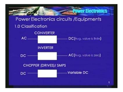
Third one: input is DC, output is also DC. Output voltage can be varied, it could be either choppers or switch mode power supplies or DC to DC converters or DC transformers.
