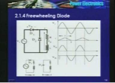
current that is flowing to the load also reduces, current slowly reduces. So, average value is same as that of a purely resistive load: in the sense, output voltage is equal to input voltage till omega t is equal to pi and beyond pi, it is 0.
