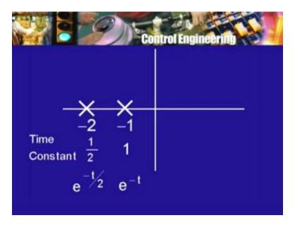
So there is no instability but in a very extreme case, the 2 poles instead being on the real axis like this which means what suppose this is minus 1 and this is minus 2, what does that mean. It
