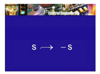
Well, in the given polynomial replace s by minus s, now what is this doing replacing s by minus s, if you think in terms of the complex plane then, it is a mapping of the complex plane which changes the flips, the plane around the j omega axis. So the positive right half plane will now become the left half plane, the left half plane will become the right half plane, the j omega axis however will remain unchanged.
