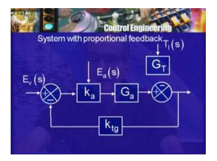
Now, when we introduce proportional feedback, the block diagram becomes modified and now, I will still show this older block diagram with the transmittances and I will show them separately. So here is plus here is minus here is this transfer function which I had called G a which is the part that multiplies E a of s and here is the transfer function G t which multiplies T l of s load
