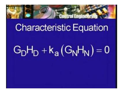
So the problem then is when I have a polynomial which looks like G D, H D plus K a in to G N, H N, what are it is going to what are going to be its roots, not for just one value of K a because we want to see the effect of the gain but when the gain is changed, what is going to happen to the roots. So, we are looking at the equation this equal to 0 or in other words, we are looking at the roots of the polynomial on the left hand side. This kind of an equation is
