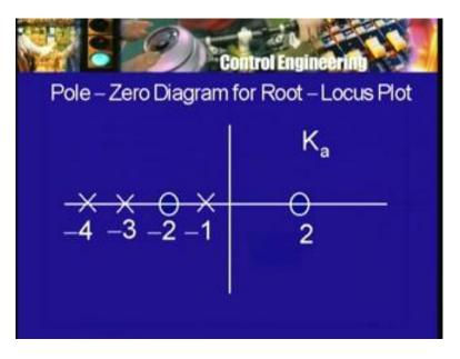
In our case, this polynomial there the characteristic equation was S plus 2 in to S plus 4 in to S plus 3 plus keeping K a and not writing 100 in to S plus 2 in to S minus 2 which results in
