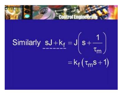
So, I have again the term s J plus k f pulling out J, I will write it as J into 1 plus 1 divided by and I will write down tau m, where tau m is the motor time constant but I can also rewrite it as k f pulling out k f as tau m s plus 1. So, we have these 2 alternate ways of writing the linear factors. One advantage of writing it this way is that, the time constant appears explicitly in one case, the motor time constant in the other case, the armature time constant.
