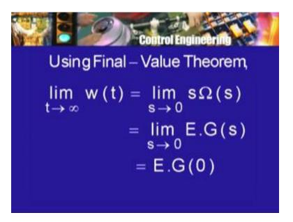
So, when I put s equal to 0 this s cancels this s cancels and I will get some expression remaining and therefore, it is that coefficient multiplied by E which will give me these steady state speed or once again the part of the steady state speed that depends on the applied voltage. So, let me write down that expression and you can go back and compare it with the expression that we had earlier.
