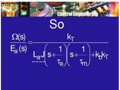
Now, the next step is to look at the transfer function once again, using this rewriting of the terms and therefore I will have the partial transfer function, omega divided by E a given by k T divided by, I have the product and now pulling out L a, I will write it as L a into s plus 1 by tau a, I also pull out J. So I will write down L a into J into s plus 1 by tau a into s plus 1 by tau m, this whole
