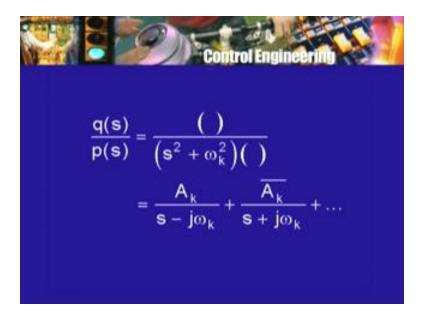
So going backwards, if in the transfer function q s by p s, if in p s I have a factor s square plus omega k squared, a quadratic factor with no s term then, it will correspond to a pair of poles like this on the imaginary axis. Therefore, in the partial fraction expansion I will have 2 terms like A k divided by s minus j omega k and A k, one can show that this will be A k bar divided by s plus j omega k, where A k will be a complex number.
