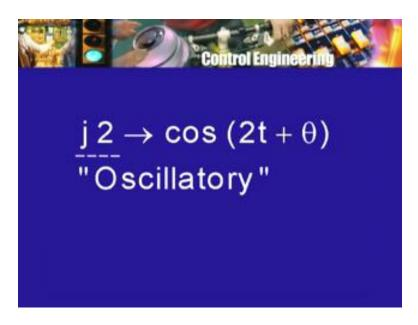
So in this case when the poles are on the j omega axis, the Laplace inverse of this part or therefore, the response will have a term which looks like A cosine omega k t plus theta k, is it good or bad. Well, it is not too bad but it may be bad because this means what, this trigonometric
