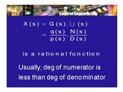
So in many cases, the Laplace transforms of the input is such that its Laplace transform is ratio of 2 polynomials n s divided by d s therefore, let me write down the expression for the part of x s that we are looking at x s is equal to G s into U s but G s is already a ratio of 2 polynomials q divided by p and U is also ratio of 2 polynomials N divided by D and so, x s is a ratio of 2
