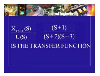
The differential equation is d square plus 5 d plus 6 operating on x equals d plus 1 operating on u, u is the input and x is the response. For this after taking Laplace transformation and looking at only one part of x of s, we got the expression that x s divided by u of s was given by s plus 1 divided by s plus 2 into s plus 3.
