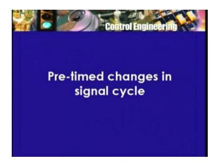
So, in the absence of such a thing, let us say somebody turns it on at 8'o clock and the timer is set for 4 hours. So for the next 4 hours, 8'o clock to 12 noon, a particular cycle of signal sequence is followed. Then, the timer goes off after the 4 hours, so another pattern then, suppose another timer is set for 4 hours, so from 12 to 4 some other pattern then, back to another pattern from 4 to 8 and then, may be a final pattern from 8 to midnight.
