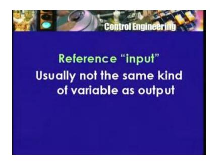
But the reference input temperature is not something real is not something which is at some 27 degrees Celsius inside the thermostat but the very setting of the bimetallic strip. There will usually be a screw of some kind there will be a spring which will push the strip down or up by some amount in the relation to the switch contact that is shows as this, the reference input, there is no physical reference input which is measured or which is stored as a physical quantity.
