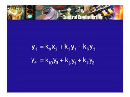
So the equation for that is Y 4 equal to K 10, Y3 plus K 5, Y 1 plus K 7, Y 2. So for each one of the 4 nodes Y 1, Y 2, Y 3, we have an equation and there are the 2 input notes X 1 and X 2 for which we have no equation, they are input nodes, there are no incoming arrows. So there is no equation and now we would like to obtain expressions for the nodes other than the inputs nodes
