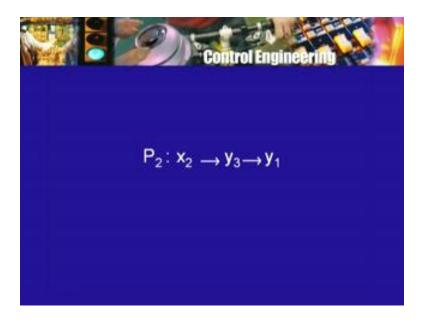
So if I want to get to Y 1, I have get to y3 first but then from y 3 can I get 2 Y 1 in some other way well from y 3 I can go to y 4 but it is seems there is no way of going to Y 1 unless I come back Y 3 from Y 3 I cannot go to Y 2. So that is it so there is only one forward path from X 2 to Y 1 and that forward path has gain K 9, K 4. Now this forward path gains K 9, K 4 is to multiplied by what remains from the delta when we remove all the loops which touch this forward path.
