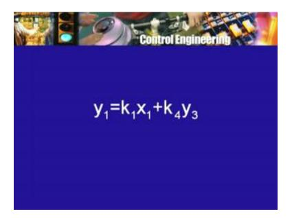
So the equation for Y 1 is Y 1 equal to K 1, X 1 plus K 4, Y 3, the equation for Y 2 it has more terms because there is K2, Y1 and there is K 8, Y 2 no, it also has only 2 terms, how about the equation of Y 3, Y 3 has 1, 2, 3 incoming arrows. So the equation for that node is Y 3 equal to K 9, X 2 plus K 3, Y 1 plus K 6 into Y 2 similarly Y 4 has 1, 2, 3 incoming edges.
