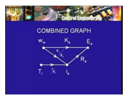
So I have T L as one node omega M as another node I A is the armature current there is that equation I have I am putting down the gains one by K T here and K F by K T there. So that is
