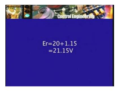
Now you can redo the calculations with a reference voltage of 21.15 K a equal to 200 as before every thing else as before and you will find out that the output speed will come out to be 1500 RPM, as is desired. So the reference voltage instead of 20 volts which corresponds to the tacho generator output voltage of 20 volts and 1500 RPM is to be a little more and how much more exactly the amount that is required to produce the desired armature voltage in this case 1.15.
