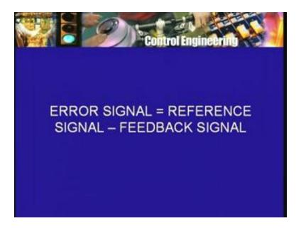
In fact, 18.85 volts will be produced by the tacho generator at a speed of about 1413 RPM. So this qualitative argument goes to show that the speed of the motor could not be 1500 RPM but then by making actual calculations with the 3 equations that we wrote down, you will find out that the speed comes out to be about 1418 RPM. So that the error voltage is about 1.09 volts and the tacho generator output voltage is 18.91 volt rather than 18.85 volts.
