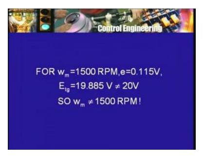
But still it cannot be exactly 1500 RPM and this is why, the books say that there will be a steady state error which is non-zero. If you increase the gain still further by another factor of 10 then the speed will be still closer to the desired speed but the point is, since you have an actual amplifier some error voltage is required to produce the output voltage of 230 volts and therefore, there will always be a steady state error that is the motor will not run at the desired speed.
