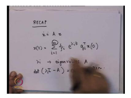
So, to make that a bit more precise, let us take a simple linear time invariant system without any input x is a vector, A is a matrix then the response of the system is given by... It is in fact a summation of several modes of course, this particular response can be written down in case you have got the A matrix diagonalizable, which we will just kind of try to understand once more.
