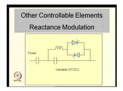
You can also you know excitation system is a simple and economic way of implementing a power system stabilizer, but you can also do other things for example, if you have got a controllable element in the system for example, this is called the thirstier controlled series compensator, essentially it is just a reactance series reactance modulation device.
