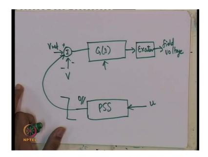
So, a damping controller or in other words a power system stabilizer has to augment the existing controller, when I say augment usually it means that you do not tamper around with the existing control system for example, if you got an AVR, so you have got a AVR, it is a exciter this is the field voltage, one possibility of course, would be try trying to augment this control system out here.
