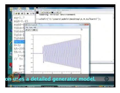
We had seen that for T m is equal to 0.8, if you give a small disturbance in V ref at time T is equal to 5 seconds a small pulse change, the system was not stable; so in fact, if you recall I had plotted the time verses power plot for this for this equilibrium condition, if I give a disturbance this system does not settle and this oscillations grows on growing with time.
