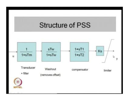
The structure of a stabilizer as mentioned before has got several important components one is of course, the limiter which ensures that the output of the PSS or the power system stabilizer does not affect the steady state regulation functions of say an excitation system. If the power system stabilizer is connected to an excitation system control like the AVR, then the power system stabilizer should not modulate the reference voltage of the AVR beyond a certain value.
