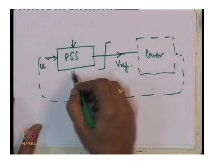
After all what you have here is an input signal and the PSS modulates something in the system for example, V ref in an automatic voltage regulator of an excitation system and this is your plant which is nothing but a power system and you got a signal which is fed back from the plant. So, this is basically a classical problem of control system design, the only catch of course, here is that the structure of the PSS has to be in some sense rather
