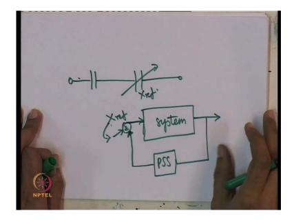
So, if you have got a series reactance modulation device, what you can do is modulate this in such a way, that it causes damping, so if you you know look at the block diagram of this it will look like this, so this is your power system stabilizer, this is your power system. This is the reactance reference of this device you sense certain signal have another, we will also call this a power system stabilizer and modulate this x ref.
