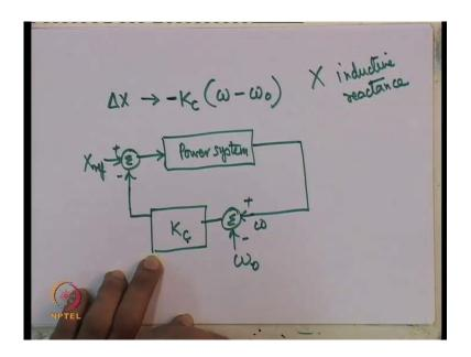
Now, the thing is that, now we have suppose delta x is modulated in proportional to I will call this some gain of the controller omega minus omega naught, so what am doing is this is your system power system, I measure the speed omega, I modulate the reactance of the transmission line by changing this, the overall reactance of the line can be changed by the react, changing the reactance of this.
