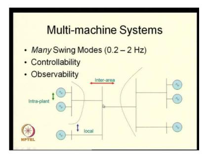
In a real life situation you may actually have many many modes, let us look at a typical multi-machine system you can have many many swing modes and one or more of these could be poorly damped or unstable. So, what you would need to do in a when designing a stabilizer of this kind would be to worry about two things, these are the two important things, which are which are important sorry, with the these are the two important things.
