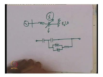
So, if for example, let me give you an example, how you could have a power system stabilizer, suppose you have got a synchronous machine connected to an infinite bus, this is an infinite bus E b angle 0 and this via transmission line which has got a controllable reactance, how do you implement this controller controllable reactance I had shown you a slide some time ago.
