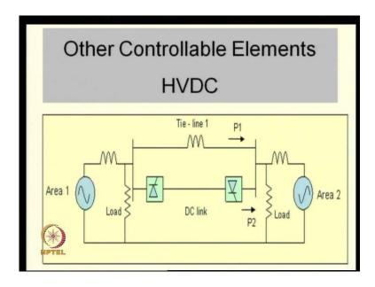
So, you will have a look at this slide, suppose you have got a two machine, two area or two machine, two area power system which looks like this, its connected by an AC line, AC tie line, it is called tie-line 1 here in this figure, and you have got a DC link in parallel as well. a DC link remembers is another controllable element in the system, you can by controlling the firing angle of the thirstier used in the convertors of an HVDC link modulate the power in a DC link.
