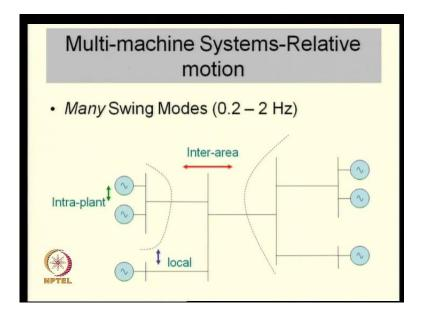
Remember that in a multi-machine system, a relative motion may be a bit more complicated than in a single machine connected to a voltage source situation, you may be having many modes of relative angular oscillations, which are depicted in this figure here.
