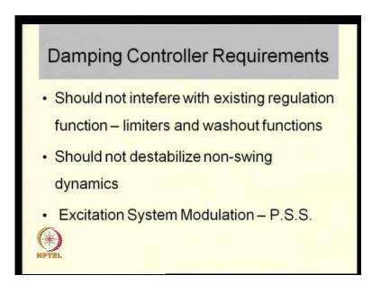
For example, the damping controller should not interfere with the existing regulation function, I mean it should not really you know compromise on the basic regulation functions which are already there for example, if you have got an automatic voltage regulator in a generator excitation system, you would like to still continue with the same function, so if any augmentation is to be done, then we should really limit that
