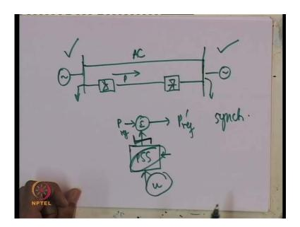
So, if you have got a two machine, two or two area system with its local load which is connected by an AC line and a parallel DC link. In that case by modulating the power in this, so you know instead of having a constant power flowing from the rectifier to the inverter, what you do is the power is modulated by another power system stabilizer, so this is P ref dash.
