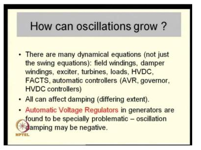
Of course, the question comes that it seems almost counter intuitive that why should oscillations grow with time? Remember that relative angular motion between synchronous machines, I discussed it by you know using a very crude crude and simple analogy of you know synchronous machines connected to each other can be considered as masses connected to each other with springs, like a multi mass, multi spring interconnected multi mass, multi spring system.
