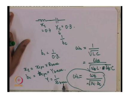
So, remember for example, in this network, you have got X 1 is equal to 0.7 in each phase and x c is equal to 0.3. So, if you look at x c is nothing but 1 by b c. So, b c is equal to 1 by 0.3.
