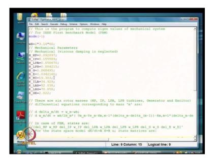
So, if you look at this program, what I have done it may not be absolutely visible on your screen. So, I will just quickly read through it, this is the data from the IEEE first bench mark model, you will assume omega is 2 point to 60 inches. So, 60 hertz system and the data corresponding to the turbine is given here, h the inertia constant value as well as the shaft constants.
