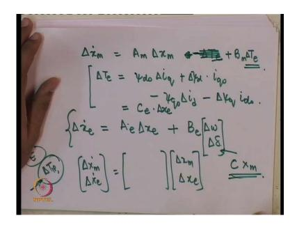
So, what you need to do, the mechanical system you will have the delta and omega variables. So, I will call them x m is equal to A m into delta x m minus delta T e. that is not going to affect all the states directly, it will affect the generator states directly. So, you actually have B matrix into delta T e and delta T e itself is equal to psi d 0 delta i q minus delta psi d into i q 0 minus psi q 0 delta i d minus delta psi q i d 0.
