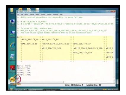
Now, this matrix is very simple. So, the states are arranged, of course, here as delta HP omega HP delta IP omega IP and so on. So, this is not required here, this part of the
