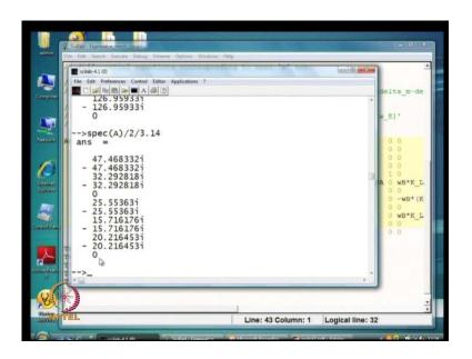
So, we will run this program, execute and form the a matrix. So, this is just forming the a matrix mechanical system. This is the mechanical system in isolation, assuming that electrical torque is not is 0 or it is a constant.
