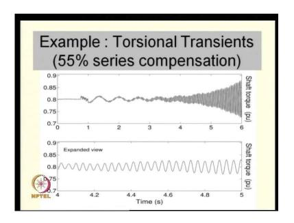
If I compensate this network by 55 percent series compensation, there is one oscillatory mode which goes unstable; this is what we find by simulating the system. Remember, if you want to simulate this phenomenon, you will have to use E m T p like programs in which stator transients and network transients are not neglected.
