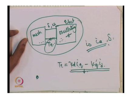
So, the point now is, you have got an electrical network, which is series compensated it has got oscillatory Eigen values or oscillatory response and the mechanical system also is in oscillatory response delta and omega T e.
