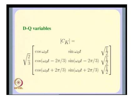
Since, we have to interface the equations of both machines, we converted the interface variables i d i q v d v q and psi d psi q using a common transformation c k. This is what we did and the algebraic equations of the network, which are supposed to be interface with the network equations.
