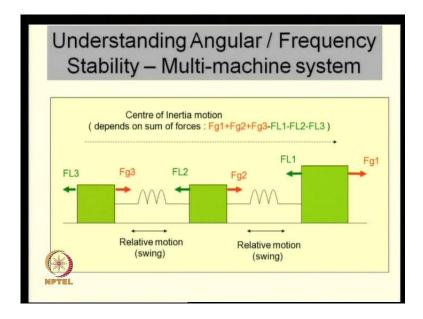
What happens when you go from one machine to three machines? So, to just kind of give a crude analogy again of a system, which is kind of a will give us at least some idea of how the electromechanical modes behave of you know whatever analogy am showing here for the spring mass system is actually, not completely does not completely reflect our system remember our system has many other modes as well.
