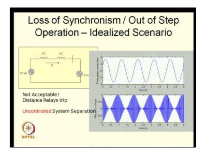
And as I mentioned sometime in case you lose synchronism that time is one set of machines has a frequency, which is tends to be different from other set of machines, then you will have oscillations, which is something we saw in the previous class, you have got oscillations in the electrical power as well as several at several places for example, in this example the midpoint voltage tends to oscillate this is a fifty hertz waveform, but you see the magnitude goes on going up and down.
