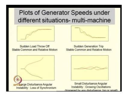
Suppose you have got this is a plot of generator speeds under various situations in a multi machine systemic of course, it is a multi machine system, but I have plotted only three machines, three speeds here this is a typical situations if there is a sudden load through off in the system the generator speeds tend to accelerate.
