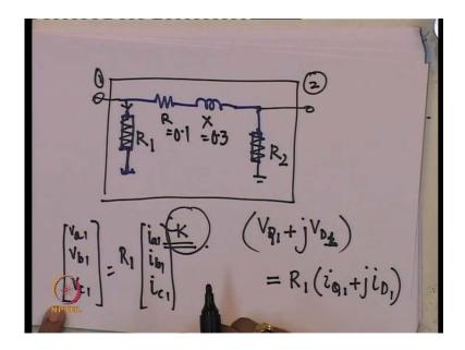
So, in this particular for example, system we have got a network like this is the load, which I mentioned sometime back was, in fact, a unity power factor load, which is of course, voltage dependent; because I have told that it is a resistive type load also. So, I assume that the load is voltage dependent it is dependent on the square of magnitude of the voltage. So, you have got a system like this, this is a network.
