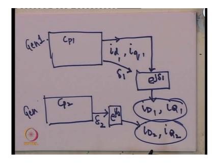
So, what really is the procedure you should apply in case you are trying to interface different generators what you need to do is you can formulate the generator equations in using C p the local frame, so you. So, from that local frame you will get i d and i q then convert this i d and i q using delta 1 to i d and i q. So, use this transformation e raised to j delta one as I mentioned here in the slide. So, can you have a look at the slide again (Refer Slide Time: 19:25).
