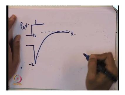
So, what you can expect is that if I give a step change in P G V the mechanical power. In fact, goes down suppose this is 0 and 1 in that case this will go down to minus 2 and then raise with the time constant of T w to 1. So, in fact I am not drawn it very well to scale.
