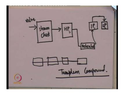
Let us talk let us discuss a common configuration in steam turbines, in common configuration is the valve determines the steam flow and the valve position in fact, and you have basically steam chest, a high pressure turbine, this is the typical configuration. The steam from the high pressure turbine is reheated pass through an intermediate pressure stage this is another turbine then there is some crossover piping and it feeds a low pressure turbine.
