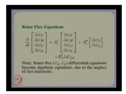
The rotor flux equations are. In fact, if you just look at these equations by themselves they are linear again, remember that stator flux is no longer the psi d and psi q are no longer states we shall see that they. In fact, obtain from the algebraic equations obtained by neglecting or setting d sci d by dt equal to 0 and d psi q by dt equal to 0 of course, A 1 dash, A 1 double dash, B 2 dash are given by these equations.
