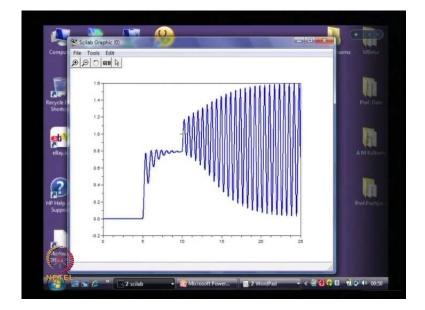
So, I have done that remember this is what we were trying to analyze. We synchronize the synchronous machine this is of course, the simulation result not the result of the Eigen analysis of course, this we synchronize the machine gave a step change in the electrical the mechanical torque then, we gave another step change to make it approximately one per unit.
