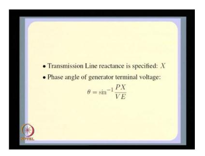
This transmission line reactance is also specified, the phase angle of the generator terminal voltage theta is computed by the formula sine inverse PX by VE. Note that in this context theta is the phase angle of the terminal voltage it is of course, a constant in steady state the reason why? I bring this to your notice is in another context we have used theta as the rotor position.
