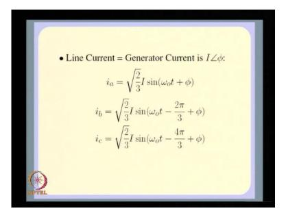
The next step is of course, getting current suppose current is I angle phi which also means i a is root 2 by 3, I sine omega is 0 t plus phi. So, if I say current is I angle phi this is what I mean are the line currents. So, this is what I mean. So, what is the value of I in such a case, if i a is related to I in this fashion then I and phi capital I and phi are given by simply this.
