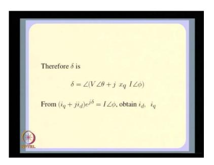
So, the point here is that because of this we can compute what the value of delta is going to be. So, once effectively what I mean to say is if you lo at the previous slide we know V angle theta plus j x q into I angle phi. So, because of that we know E f d plus x d minus x q into i d into e rise to j phi. What do I mean may be I will make it clear here.
