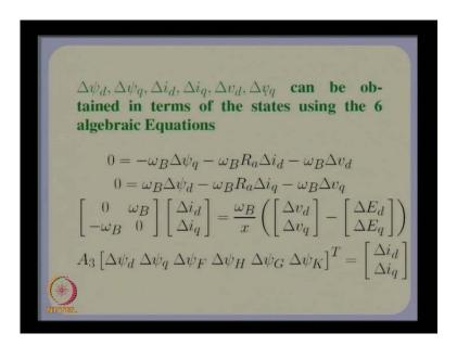
So, when you will have to when you, when you linearise it you will get delta V is equal to this. As before as discussed in the previous lecture psi d, psi q, i d, i q and V d y, V q, I can be obtained in terms these psi d, psi q, i d, i q, V d, V q appear in the differential equations, but we can actually eliminate them and write them in terms of the states using the six algebraic equations, which are linear equations these are the six algebraic equations.
