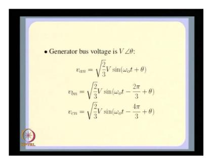
So, theta is obtained what does it mean? It means that if I get theta it means V a n, V b n and V c n are as shown. So, theta appears in this these sinusoidal terms corresponding to the voltage a to neutral b to neutral and c to neutral. So, we are assuming here of course, a star connected system, we are not considering any unbalance that is one point which you should recall. So, this is what I mean by V angle theta. So, theta is also obtained because we know the power specification.
