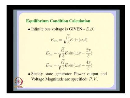
So, the first step in computing the linearized rather the equilibrium conditions is first point is the infinite bus voltage is given that is it is E angle 0 which effectively means that E a n, E B n and E c n are these this is what I mean, when I say the infinite bus voltage is E angle 0. What is specified as I mentioned some time back is that the real power output and a voltage magnitude is specified P and V.
