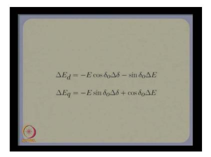
The linearized form of delta E d, E d and E q is given by these two equations remember that delta E, we assume that E is a constant. So, actually delta E is 0. So, we will just have delta E d is equal to minus  $E \cos delta 0$  into delta delta and minus delta E q is equal to minus E into sine delta 0 into delta delta.
