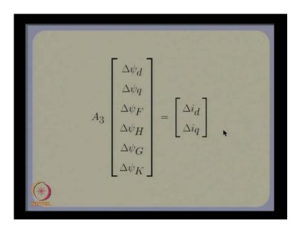
And this is the algebraic equation which relates i d and i q to the stator and rotor fluxes, where A 3 is given by this.
