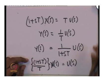
So, you will have, so what you will get eventually is, 1 plus S T of X of S is equal to t times u of S y of S is equal to 1 upon t u of S. So, from these equations what we can get effectively is, y of S is equal to 1 over 1 plus S T u of S. Is that okay? Y of S is equal to 1 plus S T upon t into u of s.
