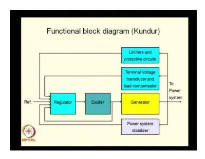
The functional block diagram of an excitation system including not only the power asperities but, also the regulators, limiters and stabilizers which effectively form the control system; remember control system is designed by us it is more of a mathematical logic which is implemented using some physical elements. So, you can have analog or
