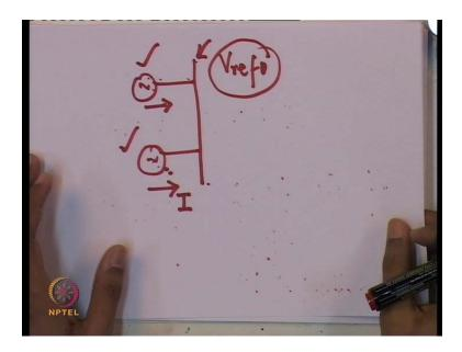
So, in both machines if I choose my K appropriately, I can actually impose a proper sharing agreement between these two generators. So, no one machine pushes in more current then what is necessary. So, what happens is that, you make the excitation system
