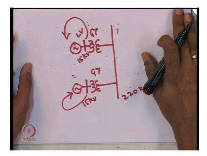
It is usually not used in situation where a common objective is not being met by two excitation system. For example, in this case when the machines are bussed together at the high voltage side and your voltage regulator is trying to maintain these voltages constant, it is not necessary to apply this load compensator and in such situations it may be absent.
