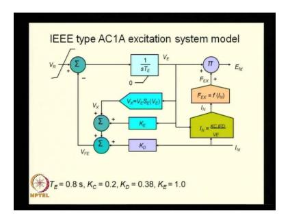
Of course, IEEE has come up with standard excitation models. In fact, the IEEE type is A C 1 A model which describes the model of a brushless excitation system is given here.
