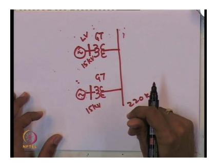
But, of course, if the generators are not bussed together; in fact, typically what happens is **heat** each generator is connected to it unit transformer. It is called a generator transformer which steps up the voltage and the generator are bussed together at the high voltage side.
