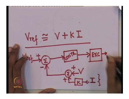
It will try to reduce. This is the exciter power apparatus, this is the controller. If this one of the generators takes on more load it tends to decrease. It will tend to decrease the final exciter voltage. And therefore, what happens is that, it prevents one generator from taking all a load. In fact, by choosing case appropriately for both machines.
