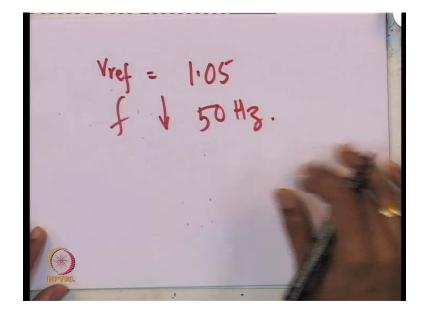
For example, if **I** given V ref 1.0 5 and you also see that the frequency of rotation of the machine has come down. It is less than normal say 50 yards hertz. The frequency has come down. In that case, the flux level in the core may be higher than what is sustainable by the core in sense the core is start heating up so and will also get saturated.
