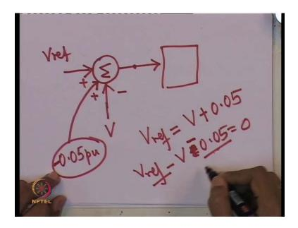
So, what you have normally is, V ref in case the generators are not bussed together right at the terminals. This is the structure of the summing point of the voltage regulator.
