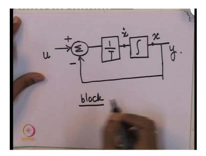
So if you look at this differential equation; I can rewrite it as a kind of integrator. This is u and this is y. This is x, x is equal to y. This is x dot. If you integrate x dot you get x dot is equal to 1 1 upon T u minus x. So, this is what exactly this says; the x dot that is d x by d t is equal to u minus x divided by T.
