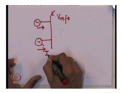
The thing is that, if you have got two machines which are connected to the same bus. So, this is two synchronous machines connected to the same bus and both these machines have an excitation system. So, both these machines have an excitation system. Both are trying to maintain the voltage of this bus a constant at V ref.
