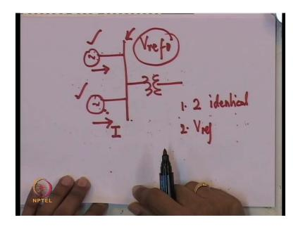
So but, in case in case two generators are bussed at common point directly, the terminals of the generator are connected to a common bus and then you step it up, side or use it for other purposes. In that case you need to have a load compensator to insure ensure that while trying to meet a common objective, the sharing of the load is done as per our design, so, this K value.
