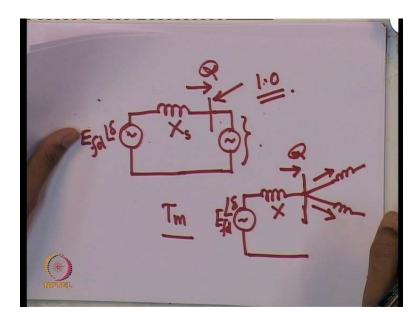
So, if you recall, a synchronous generator in its most, simplest steady state model can be represented in this fashion. This is the synchronous machine terminals. If the machine does not have saliency you can represent it by a synchronous reactant which is nothing but, equal to X d or X q because they are equal. So, this is the kind this is the steady state model of a synchronous machine.
