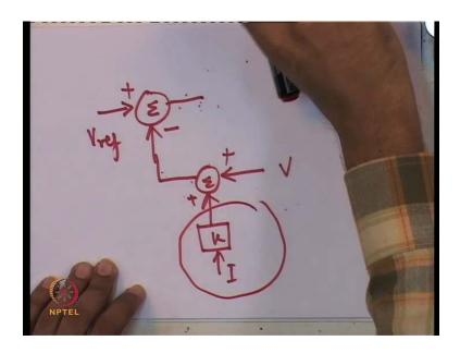
So, this particular function of V ref being modified, this summing point being modified by applying and additional correction signal here, you can say which is dependent on the loading of the machine alters the characteristic of the machine, alters the voltage. You are not may not no longer maintaining e is equal to V ref but, maintaining V plus K I approximately equal to V ref so this is called as load compensator.
