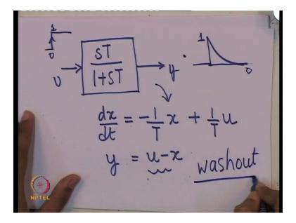
We will move on to one more Transfer function. That is, it is a kind of important Transfer function just as the previous one was. This is S T upon 1 plus S T. This is an interesting Transfer function again. You can verify that a steady state space representation of this is y is equal to u minus x. So, this is the change. So, this is a steady state representation of this system or rather states space representation of this system.
