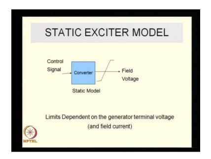
So, in the previous class we studied two kinds of excitation systems; the static excitation system whose basic model is a static one with limit's, which are determined by the generator terminal voltage. The control signal here is effectively obtained from the
