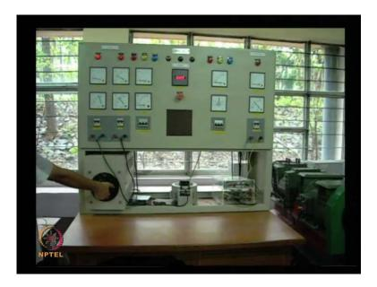
So, the machine has been started, wire the prime mover. Now, what I do is, that adjust the tool winding. Right now, there is no voltage, which there across the field. I change the delay angle of this thyristor bridge and gradually try to develop some voltage across the felid and therefore, the terminal voltage will appear. yeah So, I have a kind of try to change the delay angle.
