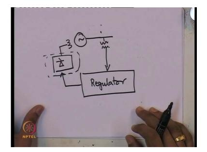
So, you measure the terminal voltages of a generator. So, what you do is of course, have a p t and feed it to a regulator. The regulator in fact, gives the appropriate signals to the control rectifier of your excitation system. It could be a brushless excitation system or static excitation system.
