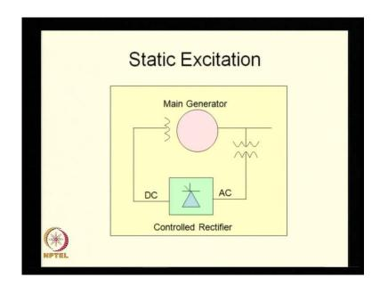
Now, the various ways of course, one can obtain the power apparatus or the the configuration of the power apparatus in order to excite the synchronous machine. Now, the major controllable element in any of this excitation system is as I mentioned some time a power electronic convertor. In fact, it is usually a Thyristor based control rectifies. So, most of the generator you will find I have got controllable element in the excitation system, which is the control thyristor bridge.
