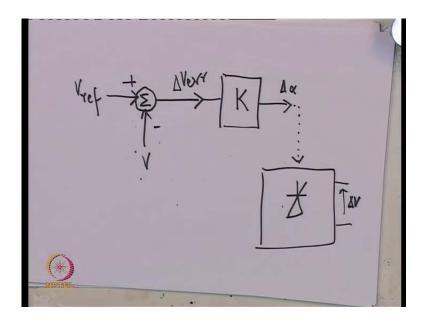
Now, what is the voltage regulator? The voltage regulator itself is some kind of control system. It is a dynamical system but it is not power apparatus. It is basically consisting of some hardware, which tries to implement certain mathematical functions. Remember, that the control signal to a thyristor bridge is not what is known as high power signal. It is just a it is has enough strength to convey to a thyristor or to the gate of the thyristors to delay there firings.
