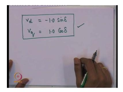
That V d by applying the transformation V d is nothing but minus 1 point 0 sine delta see, remember theta is omega naught t plus delta; so, this source has got V d and V q like this. So, recall that in our analysis of a short circuited generator, which simply put V d and V q equal to 0 and in the open circuited conditions, we assume that a very large generator very large resistance r l is connected in star at the terminals of the machine but now you are connecting it to voltage source.
