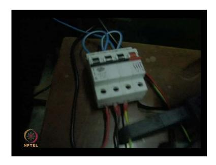
This is an MCB, which is connecting all the three phases we will be connecting all the three phases together to create a short, three phase short.
