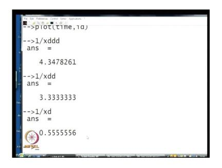
If you look at EFD which is one we have chosen it to be 1 divided by x d double dash in fact it is 4.34 which is in fact the value we are seeing here initially (Refer Slide Time: 05:33). And after some time 3.33, so you can see that, initially the current takes the value EFD by x d double dash. Then it drops very quickly and then becomes roughly EFD by x d dash and after a long time in steady state in about 2 to 3 seconds. In fact it drops down to the steady state value, which is 1 upon by x d.
