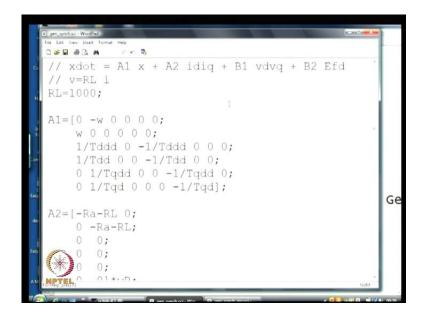
So what I have assumed is that V d and V q are related to i d and i q by this relationship v is equal to R L I R L being a very large value 1000 to simulate an open circuited generator.
