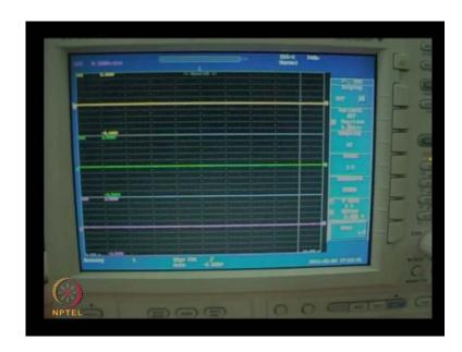
And these are the current probes, which are going to the oscilloscope at which we will observe the short circuit currents. So, now I we will actually perform the short circuit by actually connecting all the three phases together. So, the MCB will have to be switched on to the on position, and we will simultaneously view the short circuit. So, it will be any time now yeah he has given the short circuit.
