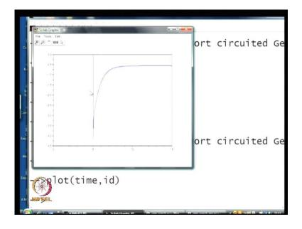
It is shown of as I said last time of the oscillatory band and in fact it goes to a value of roughly between 4 and 5 initially. Then it drops down to around 3 and then gradually drops to the steady state value. In fact what I mean will become clear here if you expand this you said that initially you see that there is a relatively sharp drop from roughly 4.25 to around 3.25 and then there is a gradual drop.
