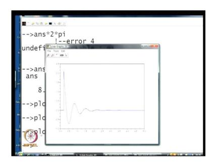
So and of course, initially the electrical torque is 0 but as soon as you connect the machine it kind of oscillates, this is a torque transient; in fact you see that the torque becomes positive and then negative and so on. And in fact it is slightly positive to begin with and then it goes negative that is one of the reason of course, is that the speed of the machine is slightly greater than that of the infinite bus.
