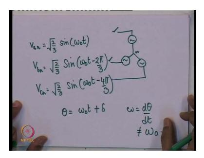
So, in fact you can you can look at this way, if **if** you have got a voltage source a star connected voltage source. So this is a star connected voltage source, it is a balanced voltage source; we will not consider 0 sequence quantities. We will assume that the voltage source is such that, V a to neutral is equal to root 2 by 3 sine omega naught t, we will assume it is a source which has got a frequency and of course, V b n is sine 2 pi by 3 a 120 degrees and V c n is root 2 by 3.
