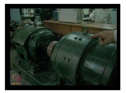
Now of course, it is not difficult to prove this it is fairly straight forward to prove that this is true, I will now show you an experimental verification of a short circuit applied on a synchronous machine. In fact we will be doing the short circuit on a medium size machine of course, this is still a small synchronous machine as compared to the machines, which are used in power systems which can go up to 100s of mega watts.
