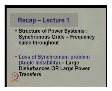
So, once we have inter connection by AC lines, we discuss this that in steady state, we ought to have frequency same throughout. It should be the same throughout the grid. One of the problems, of course, which are likely to face is that although the frequency should
