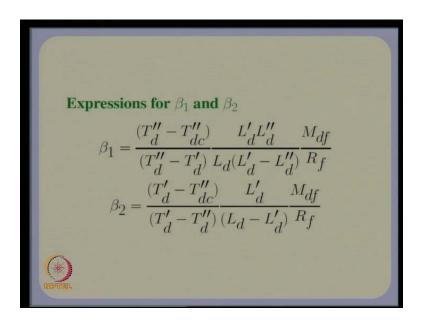
Beta 1 and beta 2, which are used in the state space model are again in terms of the standard parameters, of course, here you need to have T d c double dash, which is also a part of the transfer function which we have discussed before.
