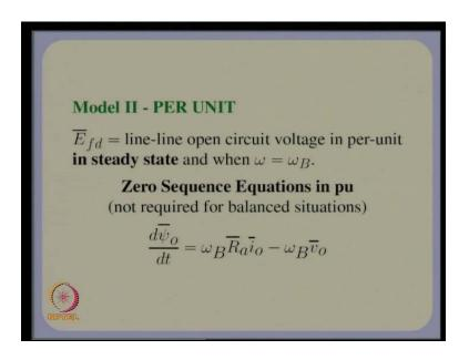
E f d bar it is a per unit value E f d bar is the line to line open circuit voltage in per unit, which would have existed or the line to line voltage which would have existed, under open circuit conditions in steady state, when the machine is rotating at omega is equal to omega B, again we have got the zero sequence equations per unit.
