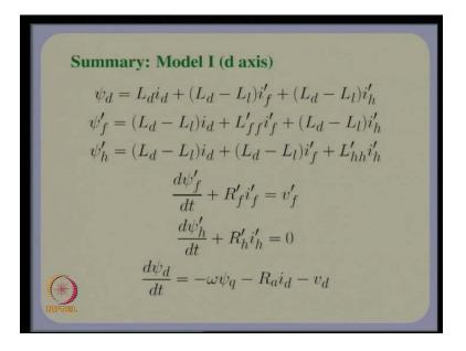
So, that is the important thing once you are back calculated the rest of the parameters you simply, you can rewrite the original model in this form; so it is a fairly straight forward kind of a a process only of course, there is one step which you have to do is, back calculate L f f the values of L f f dash, L h h dash, R f dash and R h dash, from the standard parameters using these relationships.
