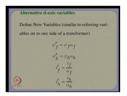
So, alpha F is in fact in some way it is a turn's ratio, alpha h is also turns ratio but, we will in fact choose it such that M d h dash is equal to M d f dash.
