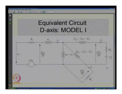
If we include the effect of the damper windings, this is what we get so we have got this now this additional branch coming here, psi d is nothing but, L l into i d plus L d minus L l into i d which is nothing but, L d into i d and since these currents i f dash and i g i h dash also getting into this psi d additionally is made out of L d minus L l into i h dash plus L d minus L l into i h dash.
