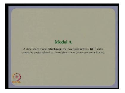
We discussed model A, which requires few parameters, in fact we use directly the standard parameters but, the states cannot be easily related to the original states, which are the stator and rotor fluxes. So, in fact we do retain the stator d and q axis flux state variables but, the rotor flux variables are not retained in this model.
