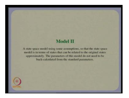
There is one important step, what I will show you is a quickly a model another model which uses a distinct approximation, this model is also useful in the sense it is going to be convenient for us to use this model, because in one step that is back calculating all parameters L h h dash, L g g dash, L k k dash and the resistances of the damper winding, that step is kind of a a rendered unnecessary if you use model II.
