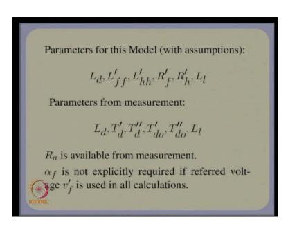
And the parameters which we get from measurement are these, alpha f is not explicitly required, if in all our calculation we use v f dash which is the referred voltage.
