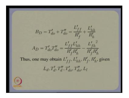
So, in this in fact in this model, we require we require of course, to obtain this model L d, L f f dash L h h dash R f dash and R h dash and L l.
