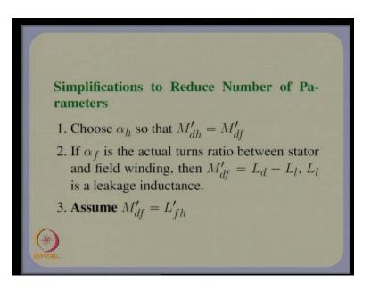
So, alpha h cannot actually be the turns ratio it is actually chosen, in a such a way that M d h dash is equal to M d f dash M d f dash is equal to L d minus L l, L l is a leakage reactance. And of course, there is a assumption made also that is M d f dash is equal to L f h dash; so we have discussed this model in the previous lecture, so I will not spend too much time on it but, the important point is that, this model uses the states psi f dash, psi h
