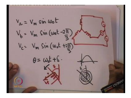
So, the a winding b winding and c winding are connected to the voltage source there is a voltage source I have got a voltage source of this kind and let us assume that this voltage source is v a v max this is a constant voltage source three phase voltage source and a balanced one that too.
