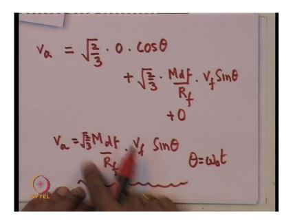
Eventually is a situation where we can find out v a from the value of v d and v q. So, what is v a from the transformation which we have defined v a is nothing, but root 2 by 3 into f v d so, v d is equal to 0 into cos theta plus root 2 by 3 into m d f by r f into v f into sine theta plus 0 so, if you have this.
