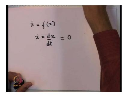
So, how do I infer the steady state behavior of a synchronous machine now the thing is that when do you say that a system x dot is equal to f of x is in steady state where x dot is equal to d x by d t we would say of course, the system is in steady state when this equals to 0 now.
