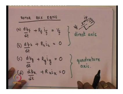
But you noticed the all the equations are time in variant theta invariant now, the rotor equations recall that we have represented the rotor as 2 coils on the d axis and 2 coils on the quadrature axis h g and k are representing the effect of damper bars as well as ready current effects in the machine.
