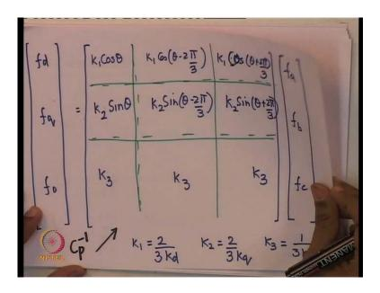
Now, the inverse transformation of course, given by this. So, the basic idea which we have tried to get is that we can do the analysis in the d q 0 variables and after obtaining the results in the d q 0 variables we try to move on and see what are the values in the a b c variables.
