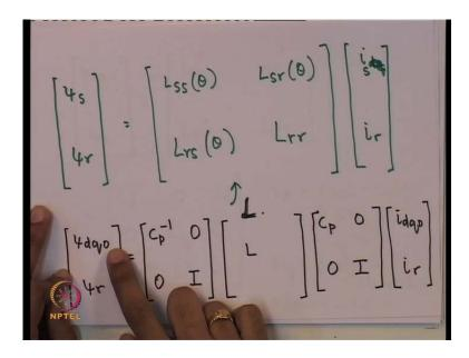
So, what I will do is apply the transformation to these variables. Remember, that the flux current relationship is psi s is equal to L ss of theta L sr of theta L ss of theta into i s into L sr of theta into i r and similarly, psi r is expressed in this fashion.
