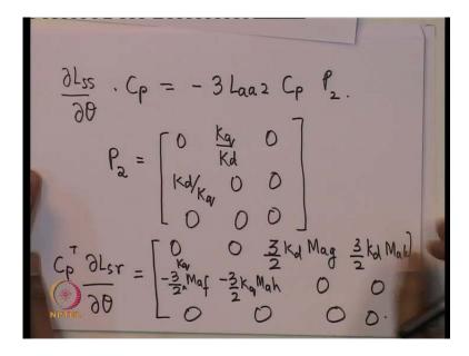
Now, you can see, that dL ss by d theta into C p is nothing, but minus of 3 L aa2 into C p into P 2, where P 2 is 0, K q by K d, 0, K d by K q, 0, 0 and 0, 0, 0. So, you can rewrite this. So, if you look at structure of d L s s by d theta if you look at the structure of it you can write it as, in this fashion.
