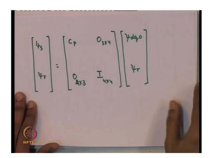
Now, the basic idea here is to convert the flux equations. So, what we will do is try to convert the a, b, c. The size, remember, is nothing, but psi a, psi b and psi c and psi R of course, is psi f, psi h, psi g and psi K psi dq. So, what we do is try to change the variables a, b, c to dq0. Of course, psi R we will keep unchanged. So, the transformation, if you look at it, is C p.
