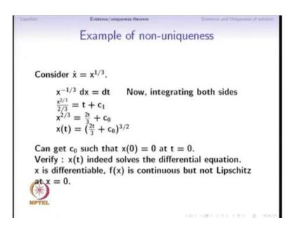
So, we see that the solution x is differentiable, we are we were able to get explicitly the solution x as a function of time we can also differentiate this as a function of time. We see that it solves this differential equation f of x is continuous, but it is not locally Lipchitz at x equal to 0. That is why the previous theorem would not guarantee existence of solutions existence and uniqueness of solutions and here is an example where uniqueness fails.
