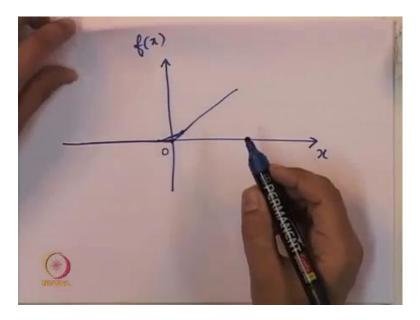
Slope between any two points, if we take the unit ramp say it is continuous. Now, so we see that the derivative does not exist at this point because the left hand limit of the derivative and the right hand limit of the derivative are not equal to each other. Hence, at the point 0, the function f is not differentiable, but we see that since the slope is bounded, we take any two points, we connect them by this line the slope is bounded, so I will just draw a bigger figure.
