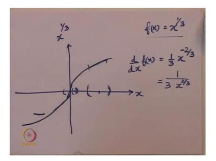
This particular graph we see that this is how the graph looks, so we see that at x equal to 0, this particular curve becomes vertical almost vertical. If we try to evaluate d by d x of
