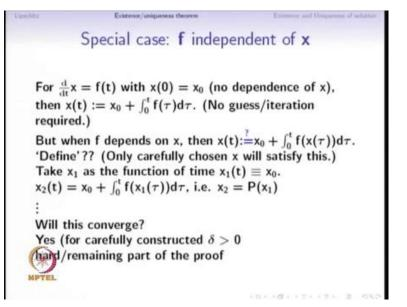
So, we will first see the special case and f is independent of x may be f is allowed to depend on time, only here we will assume that f is a function of time explicitly and there is no dependence on x. So, consider this differential equation d, d t of x is equal to f of t
