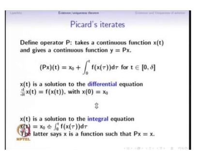
So, latter what is important is that when X satisfies this integral equation that x is also a fixed point of this operator p why because the right hand side is nothing but p of x. What x we have put in here is exactly, what is also here, that is why this particular integral equation says that p of x equal to x.
