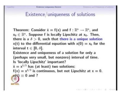
We finally come to the existence and uniqueness theorem for solution to a differential equation. So, consider x dot is equal to f of x consider this differential equation where f is a map from R n to t n and consider the point x naught in R n assume f is locally Lipchitz at z naught. Then, there is a delta greater than 0 such that there is a unique solution x of t to the differential equation to the differential equation x dot is equal to f of
