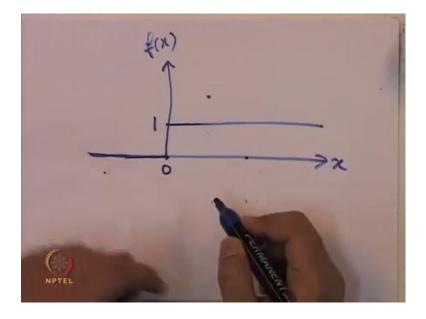
This is like our step function this is equal to 0 up to here, then suddenly it jumps to the point 1, so this particular function up to x equal t 0 it is equal to 0, for x greater than 0, it has jumped to 1. This is locally Lipchitz at every point except x equal to 0, at x equal to 0 we saw that there is this discontinuity. Hence, there will not be a constant L that will work for that inequality for all points in a ball how much ever small the ball may be.
