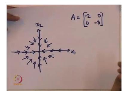
This is not the same example that is there on the slide, but it explains, what is a stable node? This is the x 1 axis this is the x 2 axis, what this says is, if we are along the x 1
