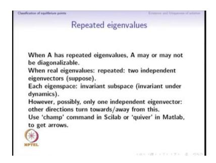
So, we have just began seeing the repeated Eigen values case. When A has repeated Eigen values A may or may not be diagonalizable, we will quickly review this part. So, when the Eigen values are repeated, then they have to be real for the case that A is 2 by 2 matrix. If they are, if the matrix A is diagonalizable then we have 2 independent Eigen vectors. Then each Eigen space is an invariant sub space, invariant meaning it is
