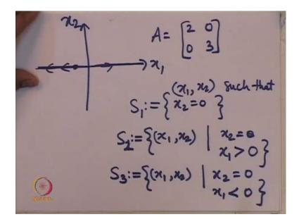
So, take the set S which is defined as all the points, where x 2 is equal to 0. The set of all points x 1, x 2 such that x 2 is equal to 0. This set is also an invariant set why because if we are along the x 1 direction because A was a diagonal matrix, x 1 axis itself being a Eigen vector. We see that the set S 1 which is defined to be the x 1 axis is also an invariant set. Of course, S x 1 axis itself contains a origin which is also an invariant set in other words another set.
