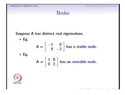
In such a situation it is called a stable node. The other situation when A has both real Eigen values and positive is called an unstable node. To analyze this, we will quickly see how the vector field looks for this particular a. So, look at this figure.
