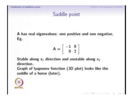
So, the situation when A has real Eigen values 1 positive and 1 negative. Again for simplicity, we will start with the diagonal case. That time because it is diagonal again we have a decoupled nature of the face portrait. So, we see because A is equal to minus 1 0 0 plus 2 along x 1 direction its approaching the origin.
