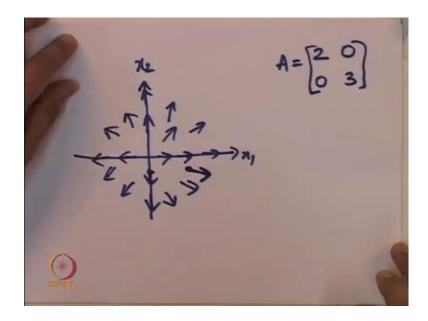
Similarly, along the x 2 axis, x 1 component is 0 and this diagonal entries being negative, imply that that is also along the x 2 axis, the arrows. The relative distance the relative length of the arrows certainly depends on the x 1 and the x 2 components, but then as far this picture is concerned as far as qualitative study is concerned this explains how the various arrows are.
