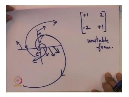
Only that the diagonal elements have positive sign. Now, all the arrows are directed away from the origin, also the rotation has been reversed because the signs of this. The previous example have been interchanged. So, here is an example where the arrows are all directed outwards. So, we have at any point we have trajectory that is going away
