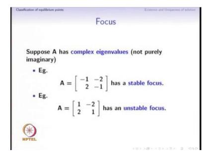
The next type of equilibrium points we will see is when a have complex Eigen values. These Eigen values are not purely imaginary. Take for example, A equal to. So, in which the diagonal elements are equal to minus 1 and the off diagonal elements have opposite signs 1 is plus 2 1 is minus 2.
