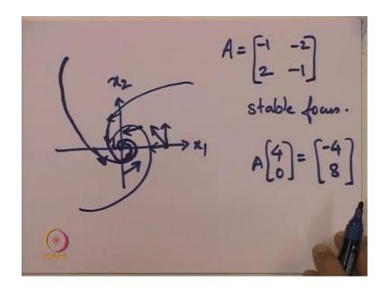
So, this we will call is a stable focus. As I said the off diagonal elements cause rotation about the origin. Each of these cases A is non-singular, hence the origin is the unique equilibrium point. So, let us take an example of a particular point and decide where the arrow is when we are at this point. So, this point for example, is 4, 0 when A acts on this we get minus 4 and below we get plus 8. So, this is a vector which is like this.
