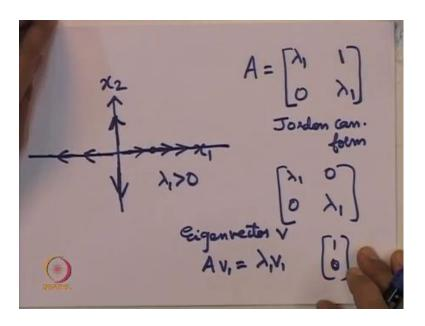
Also the situation when one or more Eigen values are at the origin. Coming back to the matrix A. When there are repeated Eigen values, that time the matrix a may or may not be diagonalizable. Say suppose we have a repeated Eigen value lambda 1 and if A is diagonalizable that is when we will like to put a 0. Here and if A is not diagonalizable, then we put a 1 this is called the Jordan canonical form, for the case when there are repeated Eigen values and a is not diagonalizable.
