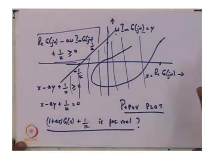
So, we make the following plot on the x axis you plot the real part of G j omega and then the y axis you plot omega times the imaginary part of G j omega. So, at any omega you evaluate the real part of G j omega it has some value let us say something and omega times the imaginary part G j omega it has some value. So, these two will give you some point there, now for each omega you evaluate this points and you plot this thing such a plot is called the Popov plot.
